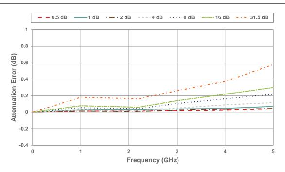
Figure 26 • 0.5 dB Attenuation Error vs Frequency
