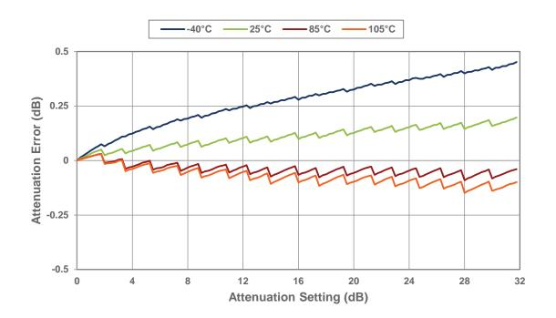
Figure 14 • Attenuation Error @ 1800 MHz vs Temperature
