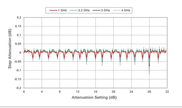
Note: \* Monotonicity is held so long as step attenuation does not cross below -0.25 dB.
