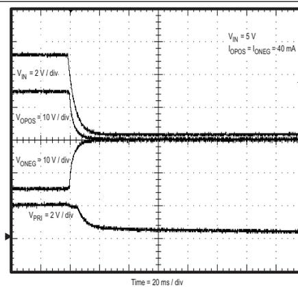
Figure 47. Power Down with Input Voltage
