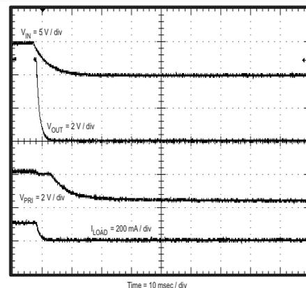
Figure 31. Power Down with Input Voltage
