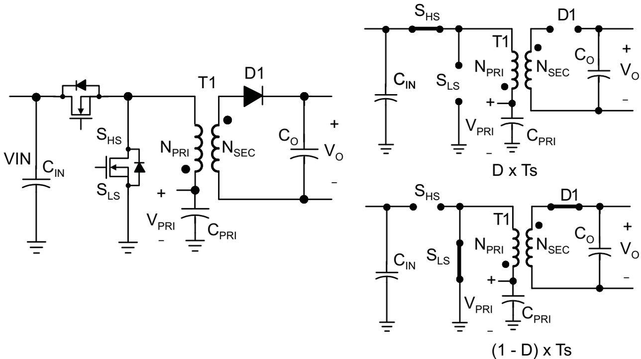
**Figure 20. Output Voltage Conversion Ratio**
