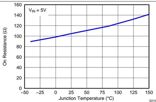
Figure 15. Fault On-Resistance vs Temperature
