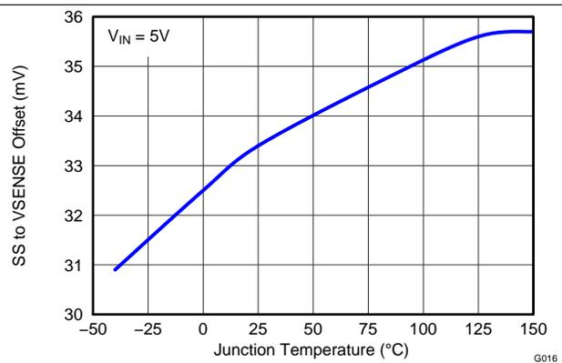
Figure 16. SS to VSENSE Offset vs Temperature
