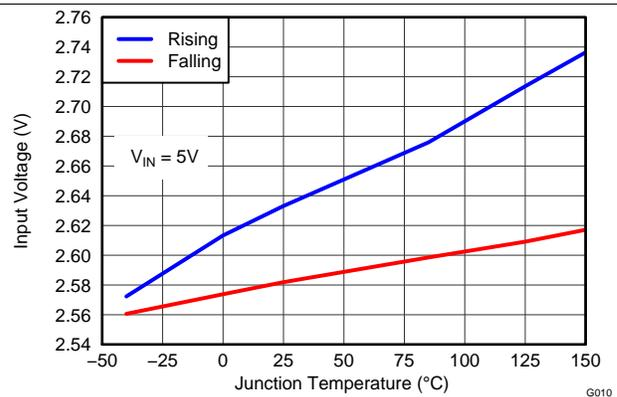
Figure 10. Input Start and Stop Voltage vs Temperature
