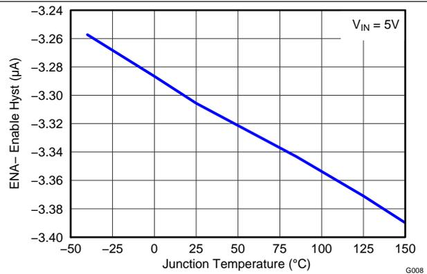
Figure 8. EN Pin Hysteresis Current vs Temperature
