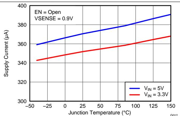
Figure 12. VIN Supply Current vs Temperature
