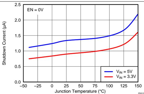
Figure 11. Shutdown Supply Current vs Temperature
