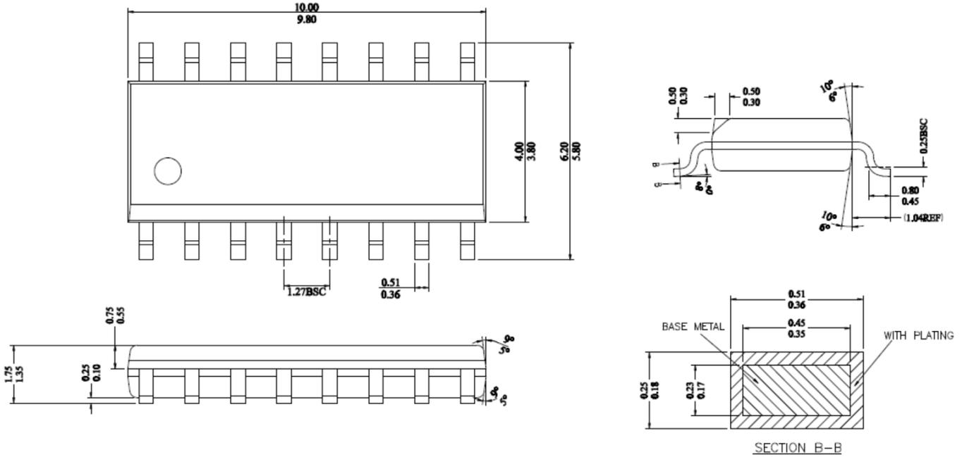
Figure18. 16-Lead Standard Small Outline Package [16-Lead SOIC\_N]
