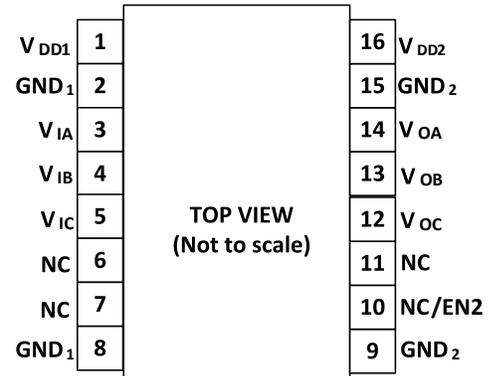
Figure3  $\pi$ 130Mxx Pin Configuration $\pi$ 131Mxx Pin Function Descriptions
