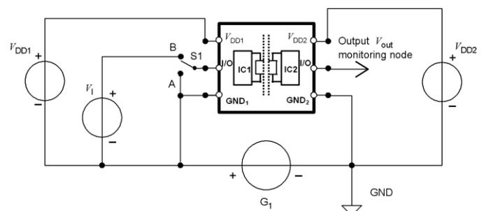
Figure 17 Common-mode transient immunity (CMTI) measurement
