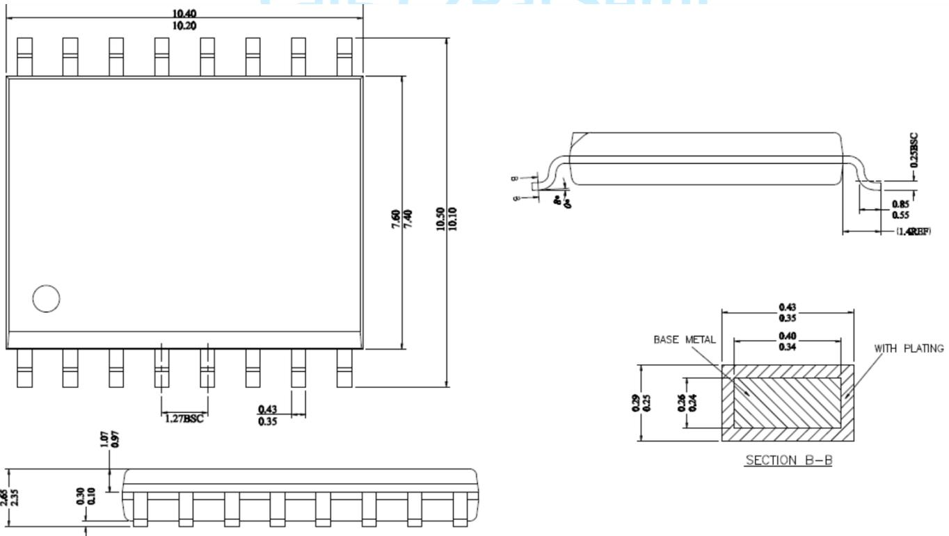
Figure19. 16-Lead Wide Body Outline Package [16-Lead SOIC\_W]
