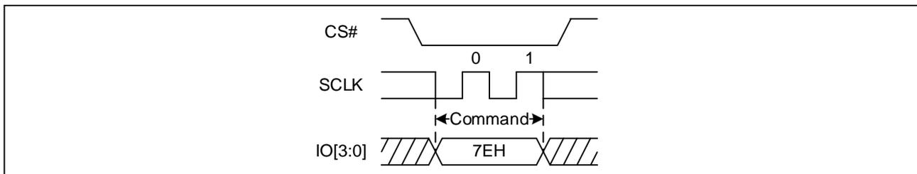
Figure 114 Global Block/Sector Unlock Sequence Diagram (SPI)
