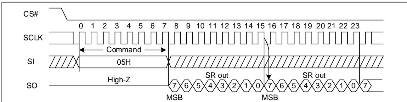
Figure 28 Read Status Register or flag register Sequence Diagram (QPI)
