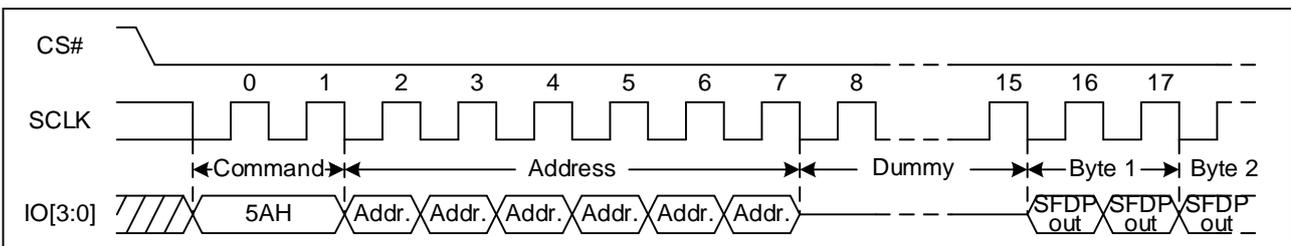
Figure 120 Read Serial Flash Discoverable Parameter command Sequence Diagram (DTR, QPI)
