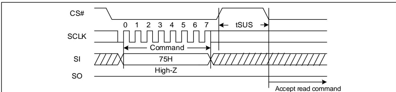
Figure 91 Program/Erase Suspend Sequence Diagram (QPI & Quad DTR)
