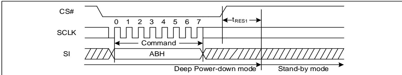
Figure 83 Release Power-Down Sequence Diagram (QPI & Quad DTR)
