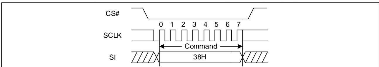
Figure 78 Enable QPI mode command Sequence Diagram (Quad DTR)
