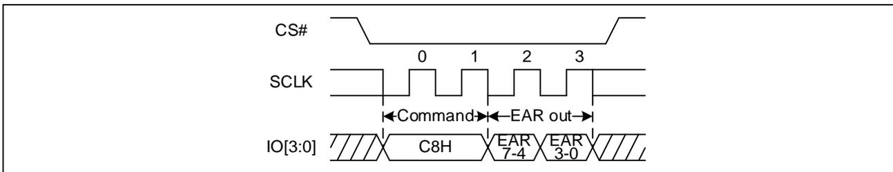
**Figure 38 Read Status Register or flag register Sequence Diagram (Quad DTR)**
