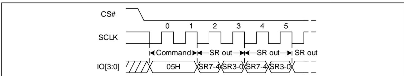
Figure 29 Read Status Register or flag register Sequence Diagram (Quad DTR)
