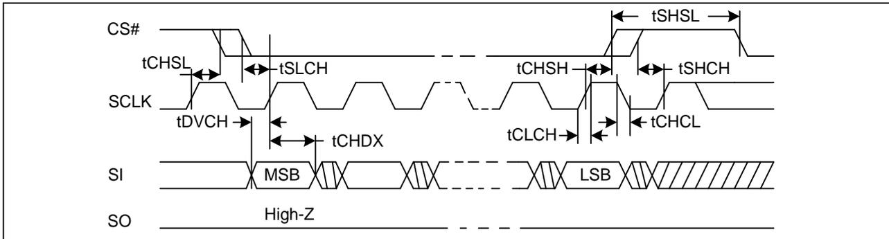
Figure 125 Output Timing
