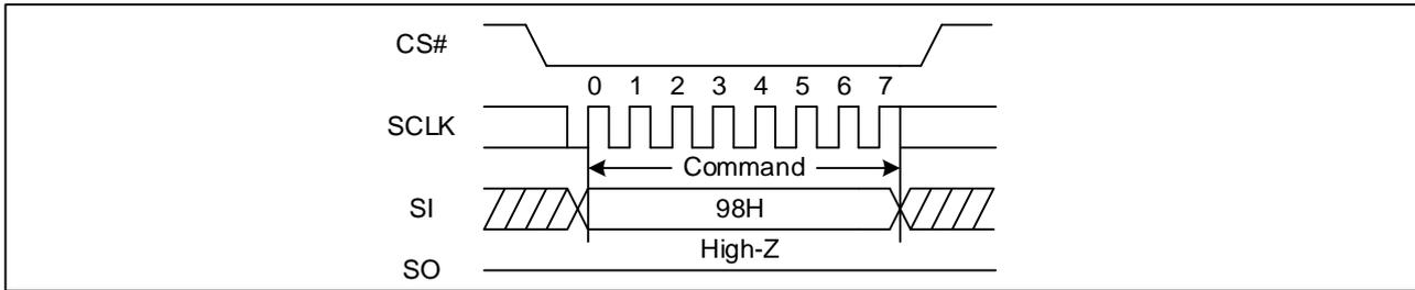
Figure 115 Global Block/Sector Unlock Sequence Diagram (QPI & Quad DTR)
