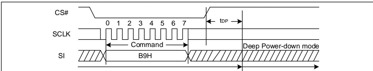
**Figure 81 Deep Power-Down Sequence Diagram (QPI & Quad DTR)**
