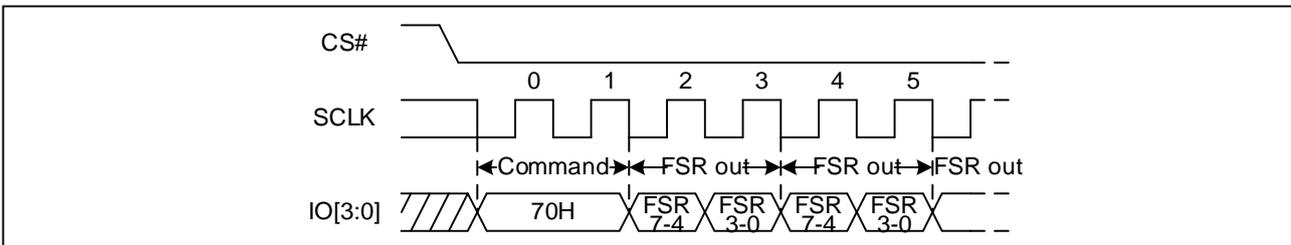
Figure 32 Read Status Register or flag register Sequence Diagram (Quad DTR)
