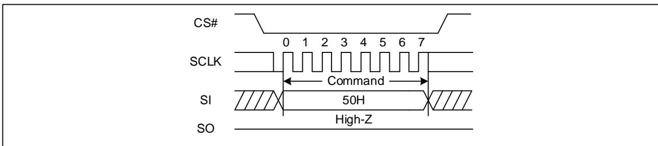
Figure 17 Write Enable for Volatile Status Register Sequence Diagram (QPI & Quad DTR)
