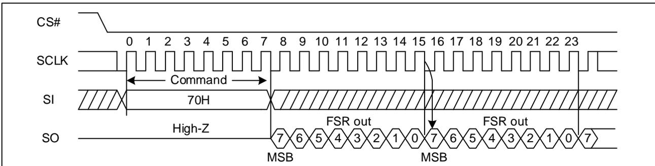
Figure 31 Read Status Register or flag register Sequence Diagram (QPI)
