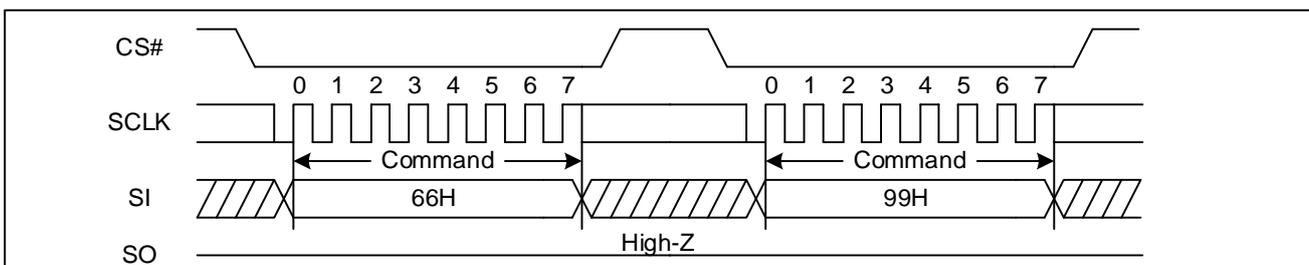
Figure 117 Enable Reset and Reset command Sequence Diagram (QPI & Quad DTR)
