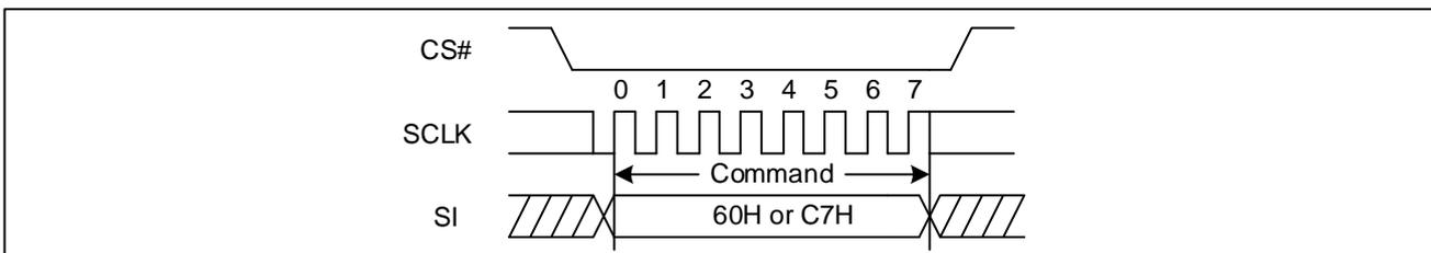
Figure 74 Chip Erase Sequence Diagram (QPI & Quad DTR)
