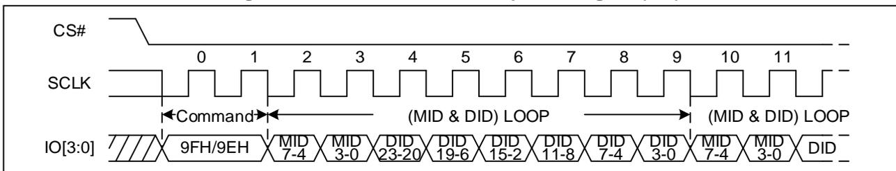
Figure 89 Read Identification ID Sequence Diagram (Quad DTR)
