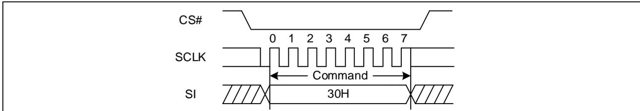
Figure 76 Clear Status Register Flags Sequence Diagram (QPI & Quad DTR)
