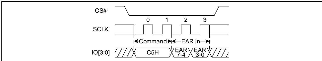
Figure 23 Write Extended Register Sequence Diagram (DTR, QPI)
