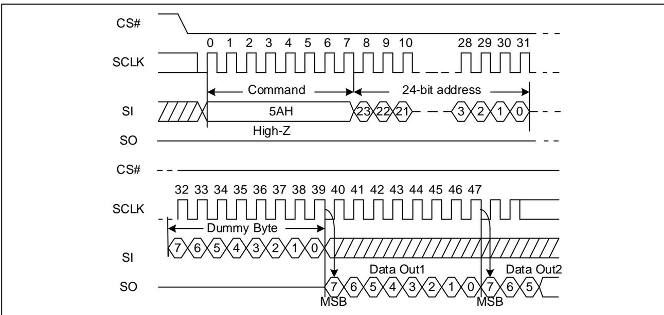
Figure 119 Read Serial Flash Discoverable Parameter command Sequence Diagram (QPI)
