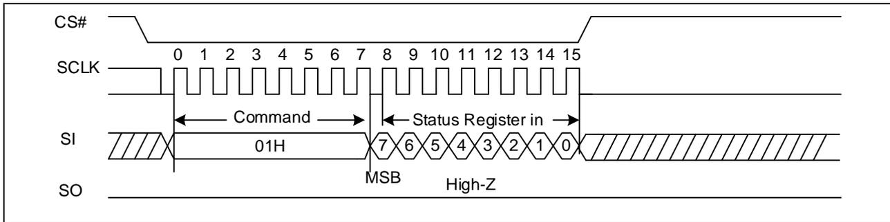
Figure 19 Write Status Register Sequence Diagram (QPI)
