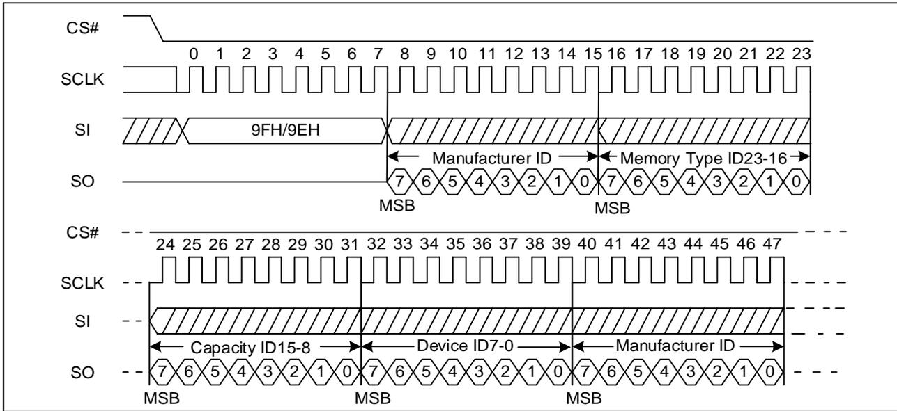
Figure 88 Read Identification ID Sequence Diagram (QPI)
