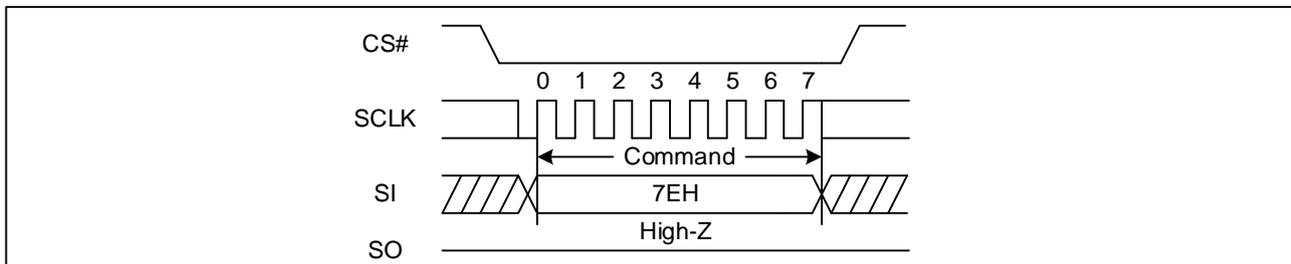
Figure 113 Global Block/Sector Lock Sequence Diagram (QPI & Quad DTR)
