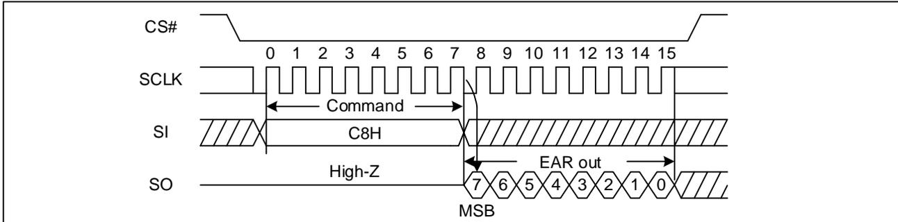
**Figure 37 Read Extended Address Register Sequence Diagram (QPI)**
