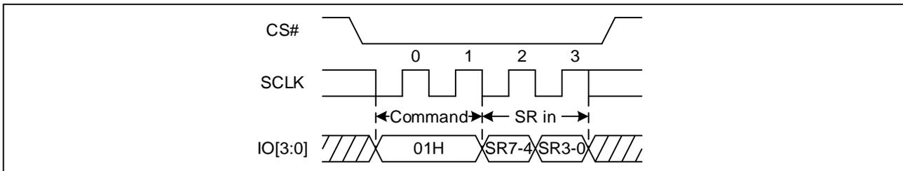
Figure 20 Write Status Register Sequence Diagram (Quad DTR)
