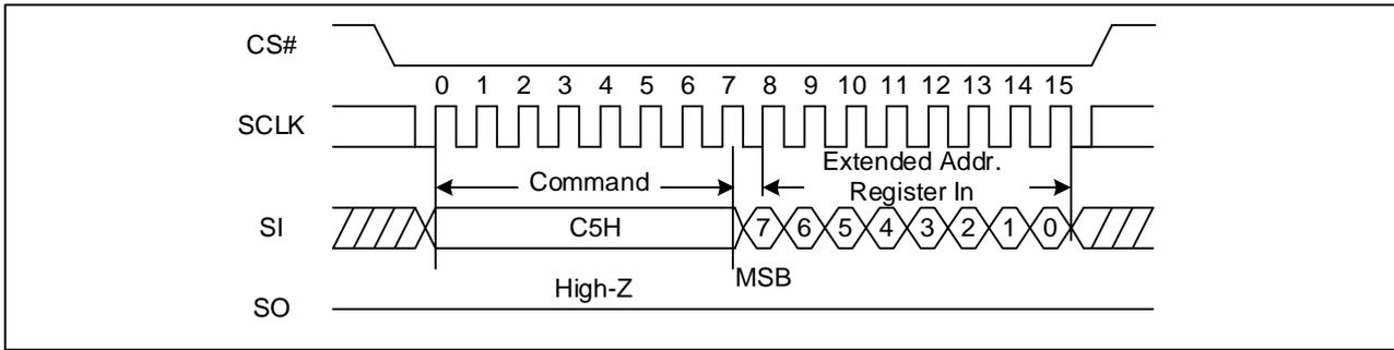
Figure 22 Write Extended Address Register Sequence Diagram (QPI)
