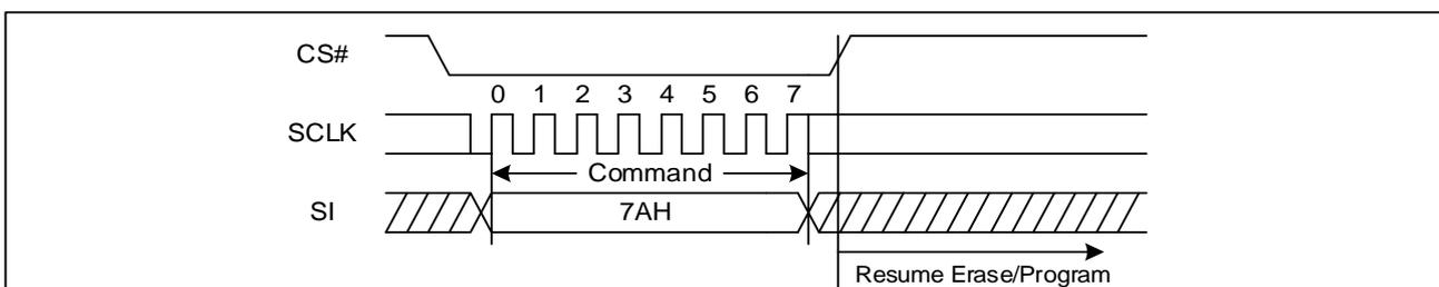
**Figure 93 Program/Erase Resume Sequence Diagram (QPI & Quad DTR)**
