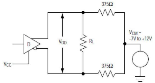
Figure 2. Driver  $V_{OD}$  with Varying Common-Mode Voltage
