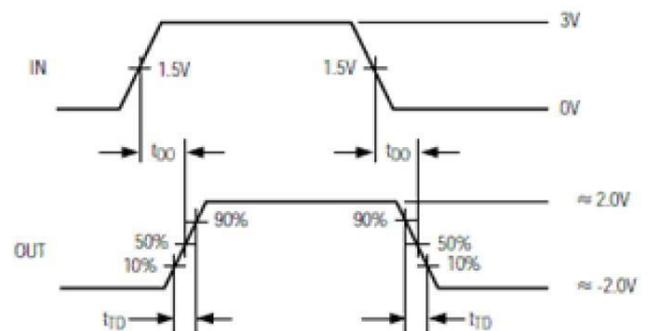
Figure 4. Driver Differential Output Delay and Transition Times
