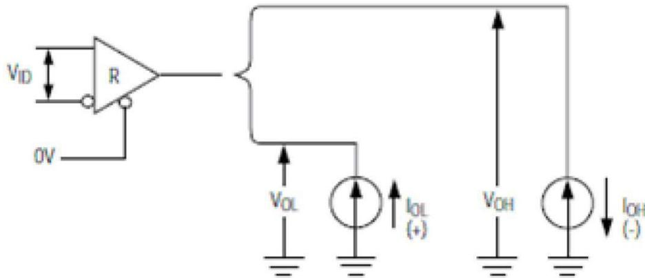
Figure 3. Receiver  $V_{OH}$  and  $V_{OL}$
