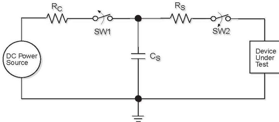
Fig. 1 ESD Test Circuit for Human Body Model
