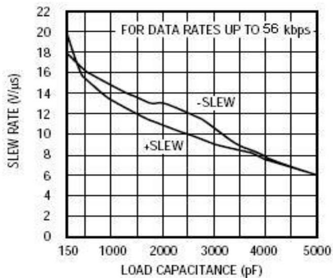
SLEW RATE vs. LOAD CAPACITANCE
