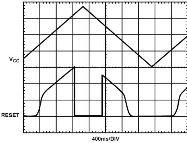
Figure 7. RESET Output Voltage vs. Supply Voltage
