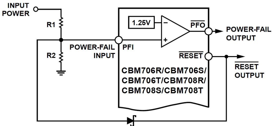
Figure 17. Power Fail Comparator
