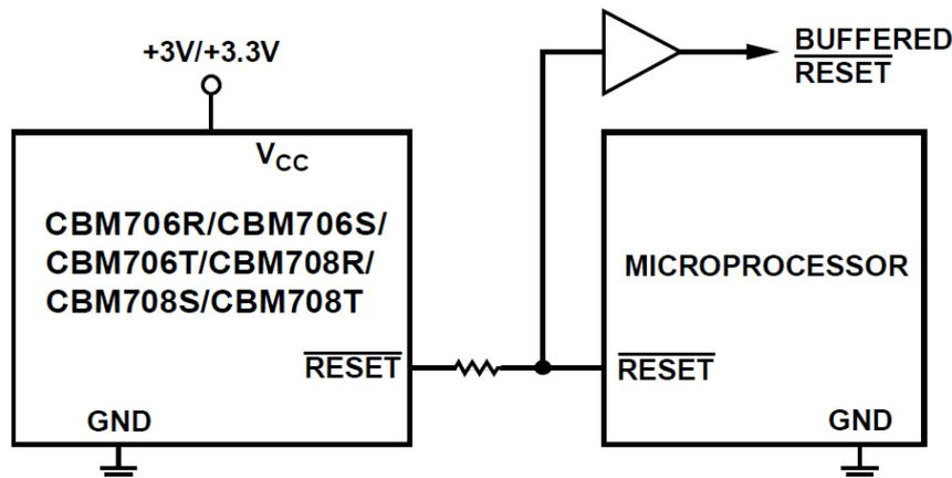
Figure 23. Bidirectional Input/Output RESET
