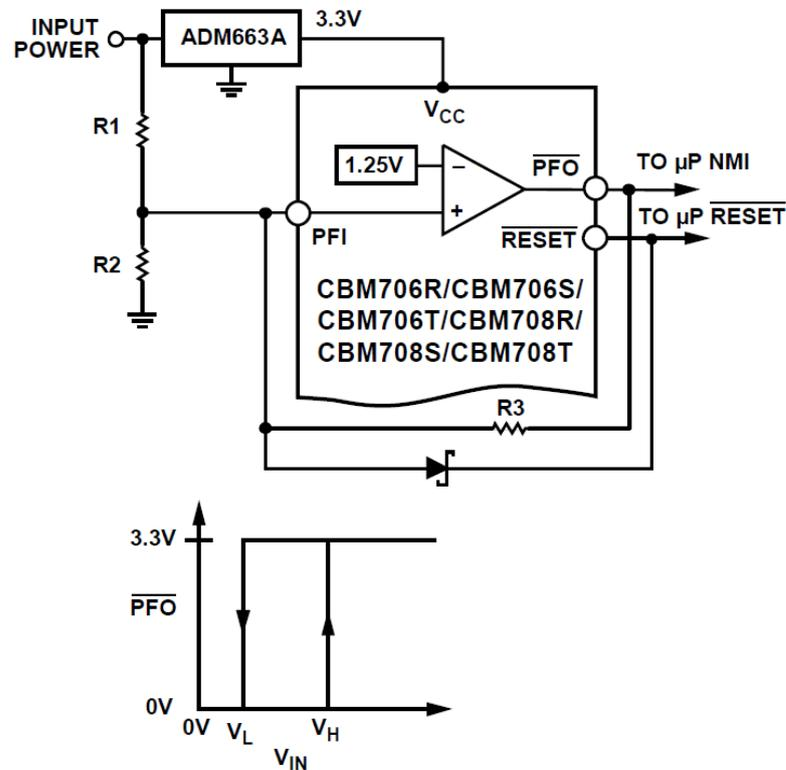
Figure 18. Adding Hysteresis to the Power Fail Comparator
