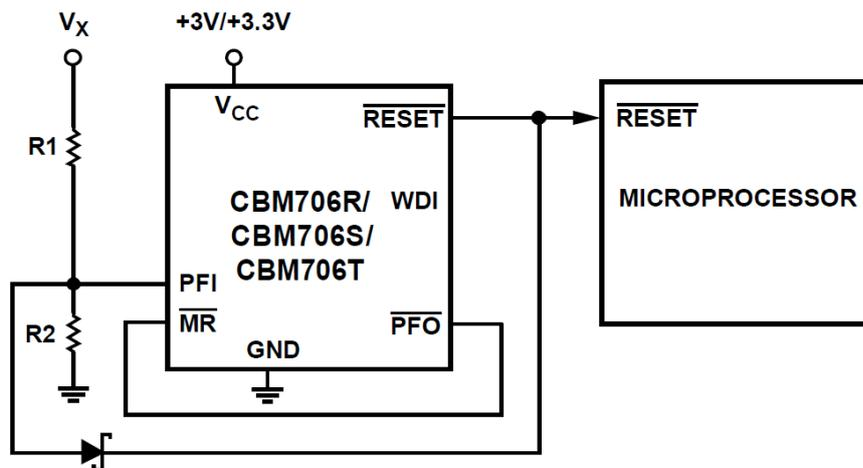
Figure 22. Monitoring 3 V/3.3 V and an Additional Supply, V<sub>x</sub>
