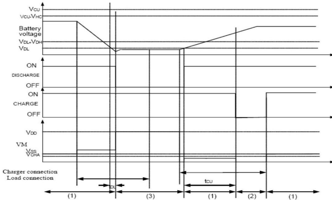
Notes: (1) Normal condition (2) Overcharge voltage condition (3) Overdischarge voltage condition (4) Overcurrent condition
