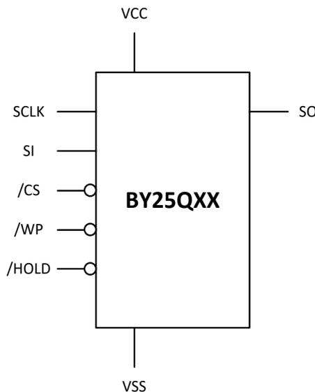
Figure 2. Pin Configuration SOP 208 mil
