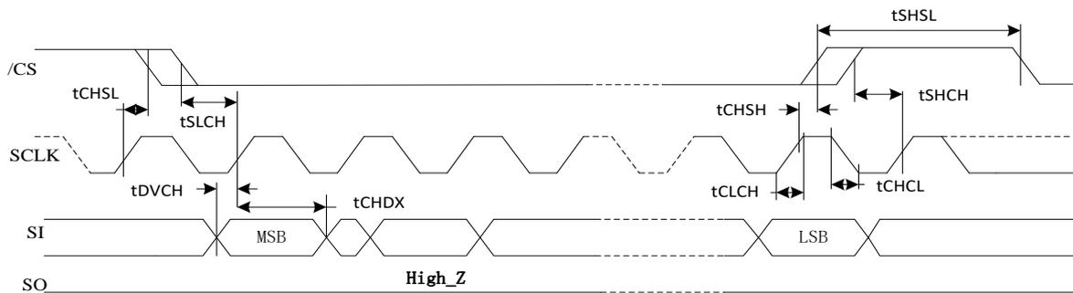
Figure 47. Output Timing
