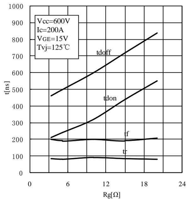
Fig.8 Typ. Switching Times vs. Gate Resistor Rg
