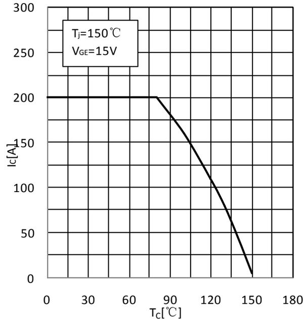
Fig.12 Rate Current vs. Temperature ( $T_c$ )
