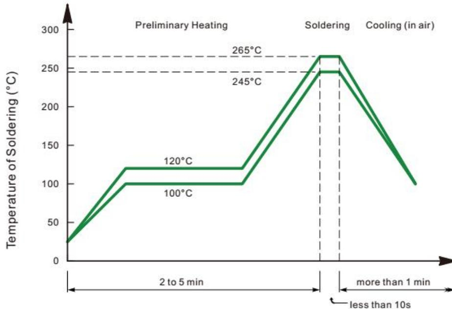
• Recommended condition of reflow soldering
