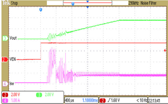
Start UP & Inrush Current 12V→3.3V (Load 1A)
