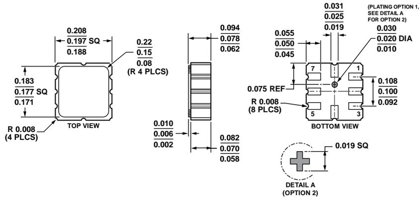
Figure 23. 8-Terminal Ceramic Leadless Chip Carrier [LCC]
