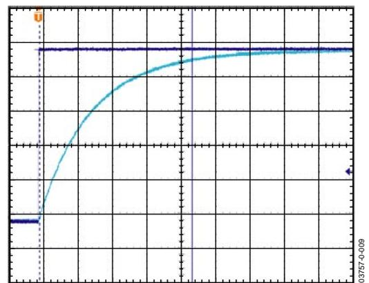
Figure 20. Turn-On Time – C<sub>X</sub>, C<sub>Y</sub> = 0.1 µF, Time Scale = 2 ms/div
