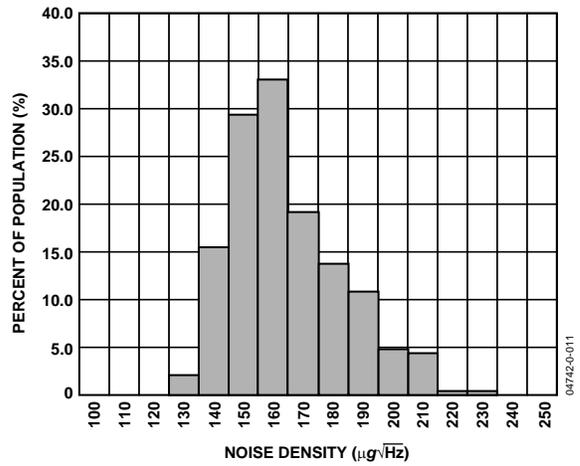
Figure 13. Y Axis Noise Density at 25°C
