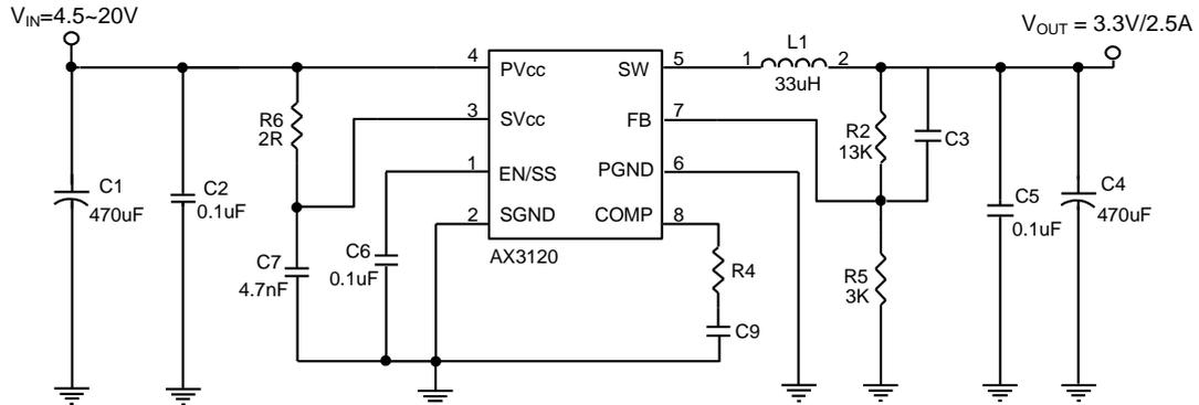
$$V_{OUT} = V_{FB} \times \left(1 + \frac{R2}{R5}\right)$$
