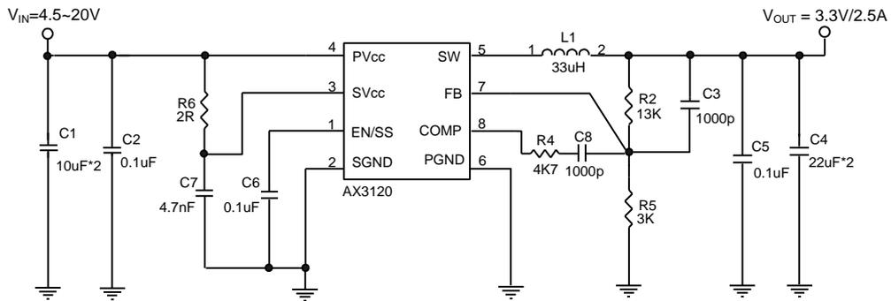
$$V_{OUT} = V_{FB} \times \left(1 + \frac{R1}{R5}\right)$$
