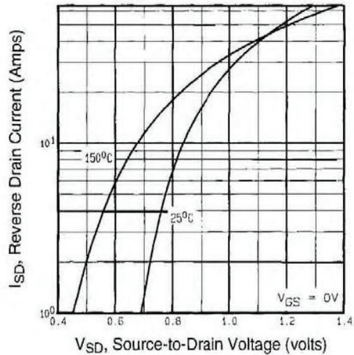
Fig. 7 - Typical Source-Drain Diode Forward Voltage
