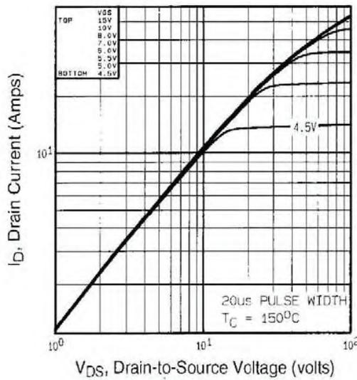
Fig. 2 - Typical Output Characteristics,  $T_C = 150\text{ }^\circ\text{C}$
