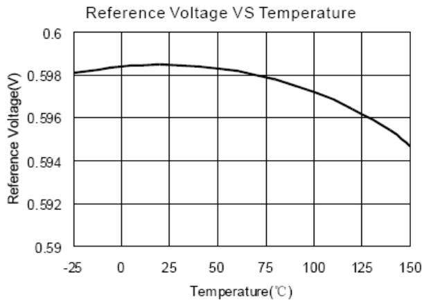
**Typical Performance Characteristics** (cont.) (@ $T_A = +25^\circ\text{C}$ ,  $C_{IN} = 10\mu\text{F}$ ,  $C_O = 10\mu\text{F}$ ,  $L = 4.7\mu\text{H}$ , unless otherwise specified.)
