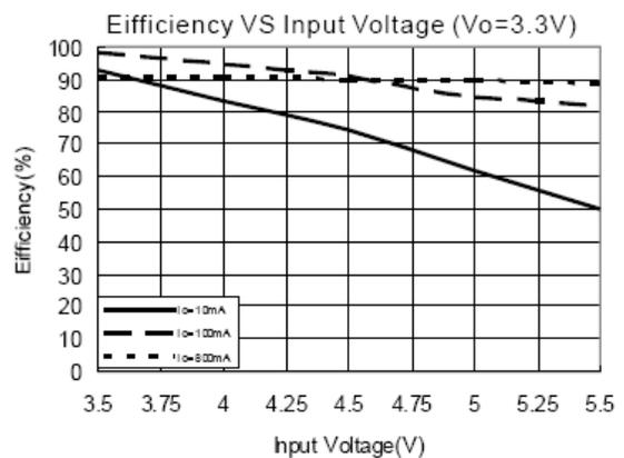
**Typical Performance Characteristics** (cont.) (@ $T_A = +25^\circ\text{C}$ ,  $C_{IN} = 10\mu\text{F}$ ,  $C_O = 10\mu\text{F}$ ,  $L = 4.7\mu\text{H}$ , unless otherwise specified.)
