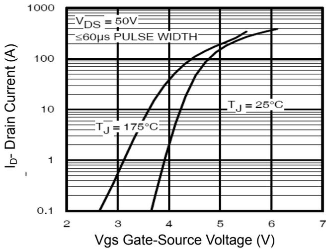
Figure 2 Transfer Characteristics
