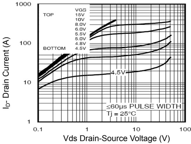
Figure 1 Output Characteristics
