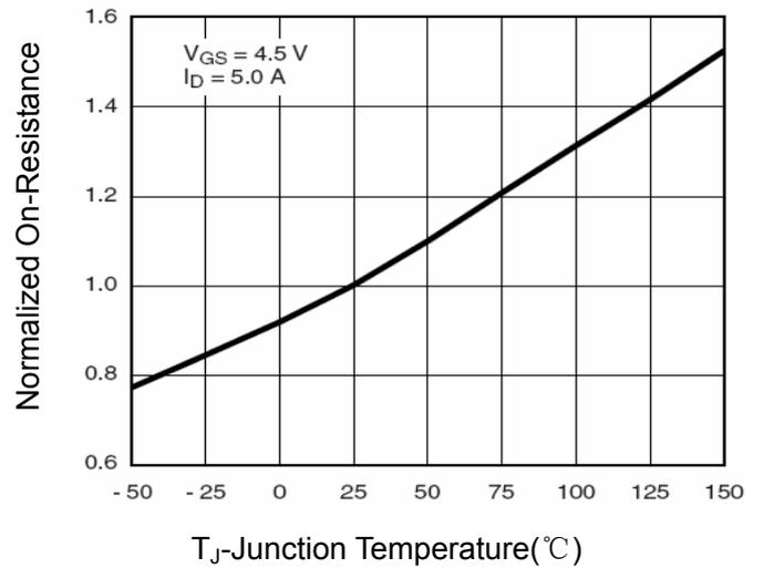
Figure 8 Drain-Source On-Resistance
