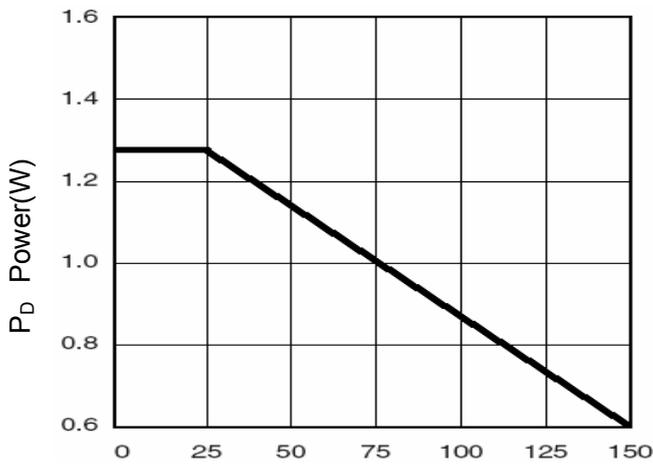
Figure 3 Power Dissipation
