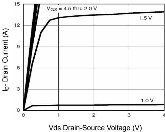
Figure 5 Output Characteristics
