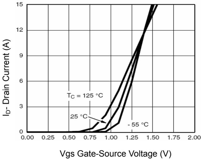
Figure 7 Transfer Characteristics
