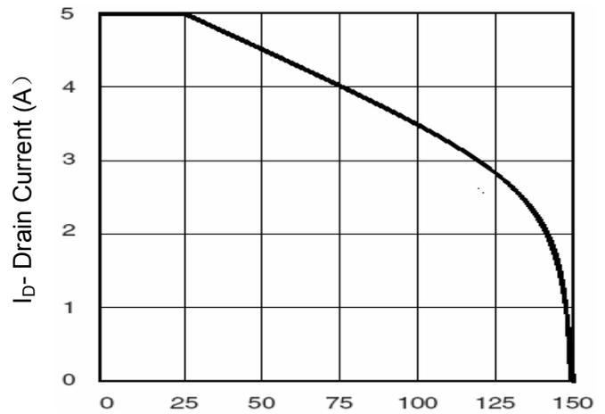
Figure 4 Drain Current
