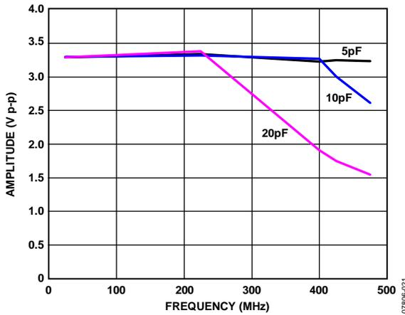
Figure 10. Peak-to-Peak Output Voltage vs. Frequency, CMOS
