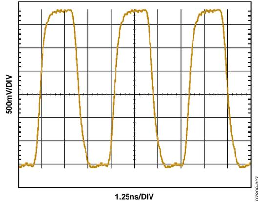
Figure 16. Typical Output Waveform, CMOS (250 MHz, 15 pF Load)
