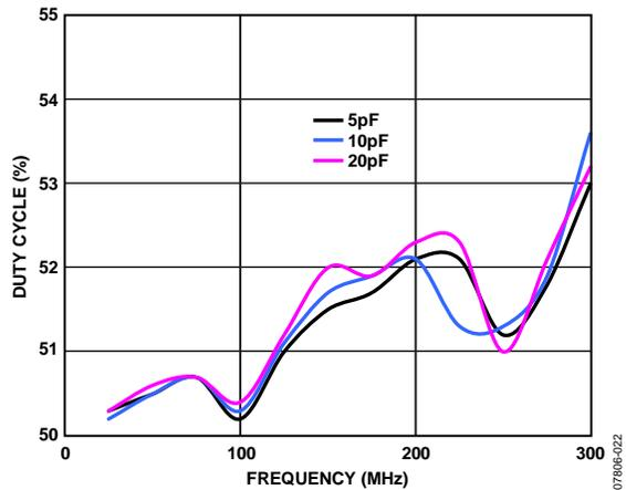
Figure 11. Duty Cycle vs. Output Frequency, CMOS
