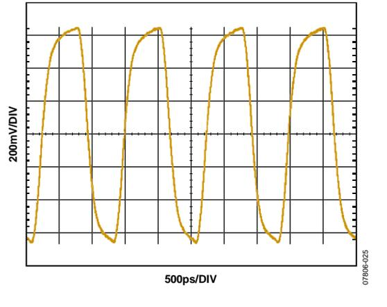
Figure 14. Typical Output Waveform, LVPECL (805 MHz)
