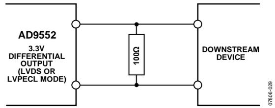
Figure 18. DC-Coupled LVDS or LVPECL Output Driver
