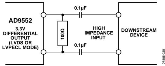
Figure 17. AC-Coupled LVDS or LVPECL Output Driver
