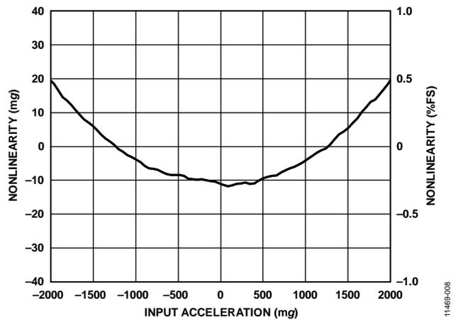
Figure 8. Z-Axis Nonlinearity,  $\pm 2$  g Input Range
