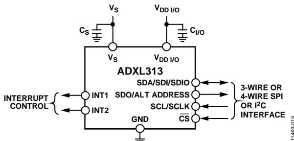
Figure 23. Application Diagram
