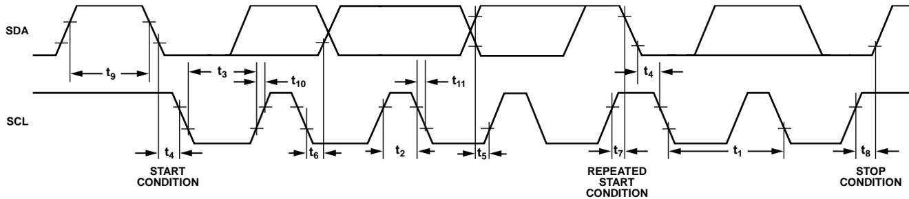
Figure 22. I<sup>2</sup>C Timing Diagram
