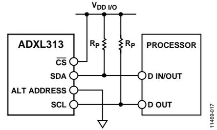
Figure 20. I<sup>2</sup>C Connection Diagram (Address 0x53)
