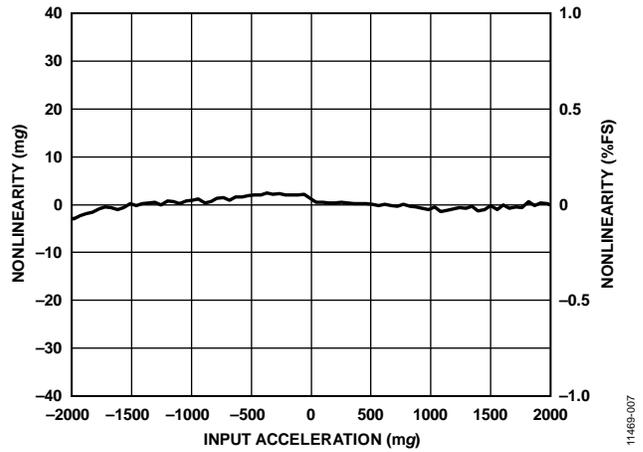
Figure 7. Y-Axis Nonlinearity,  $\pm 2$  g Input Range
