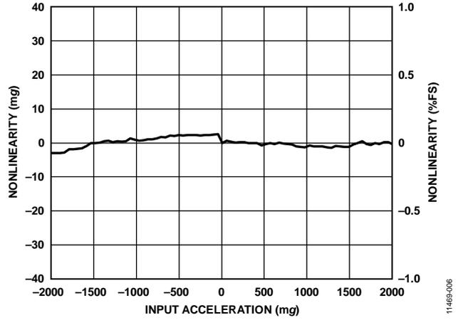
Figure 6. X-Axis Nonlinearity,  $\pm 2$  g Input Range
