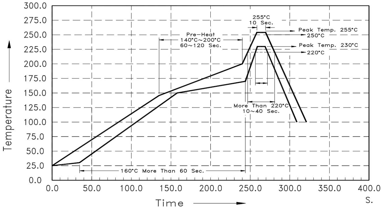
The Profile is available that must to use SnAg<sub>(x=3.3~3.8)</sub> Cu<sub>(y=0.2~0.7)</sub> solder paste
