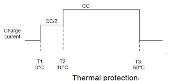
The NTC feature is implemented using an internal 48µA current source to bias the thermistor connected from the NTC terminal to GND(designed for use with a 10k NTC  $\beta = 3370$  [SEMITEC 103AT-2 or Mitsubishi TH05-3H103F]). If NTC feature is not needed, a fixed 10kΩ can be placed between NTC and GND to allow normal operation. Since the  $I_{NTC}$  current is fixed along with the temperature thresholds, it is not possible to use thermistor values other than the 10k NTC (at 25°C).
