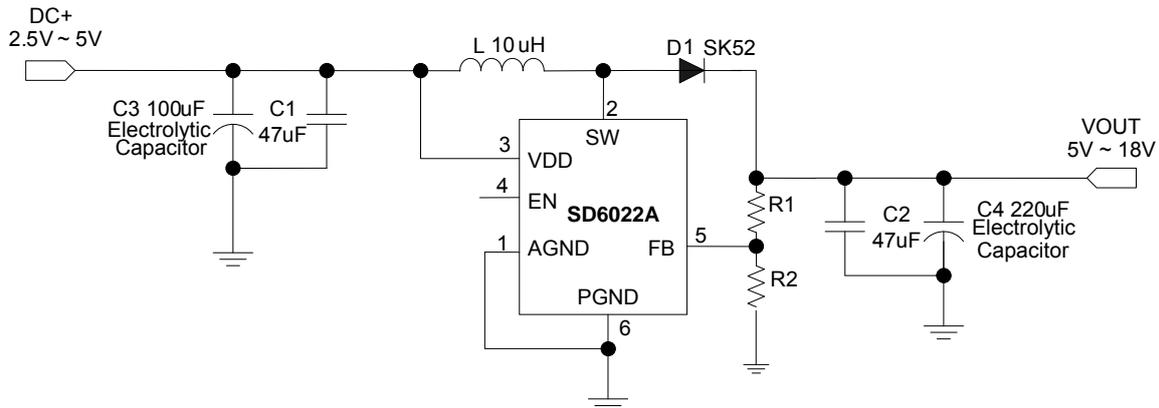
\* The Output voltage is set by R1 and R2:  $V_{OUT} = 1.212V \cdot [1 + (R1/R2)]$
