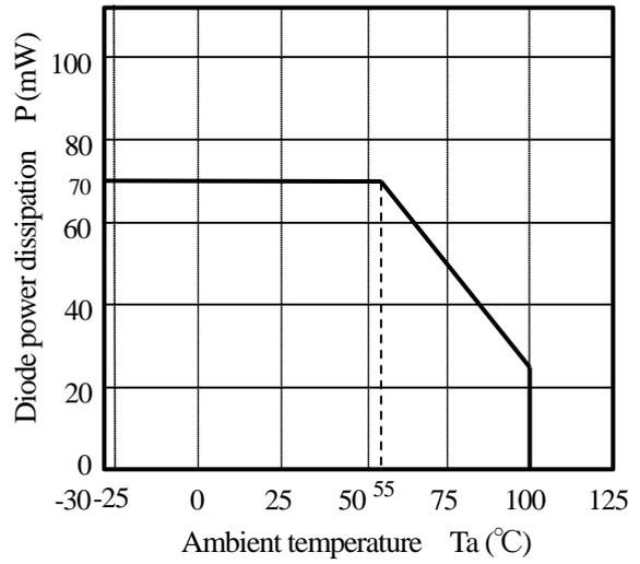
(Fig. 3) Collector power dissipation vs. Ambient temperature
