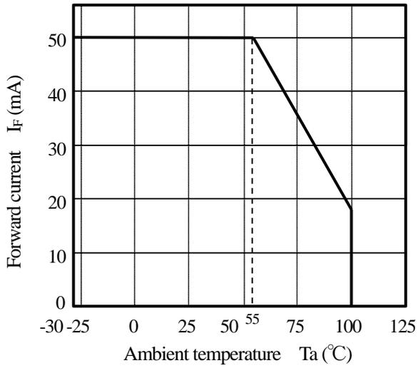
(Fig. 2) Diode power dissipation vs. Ambient temperature
