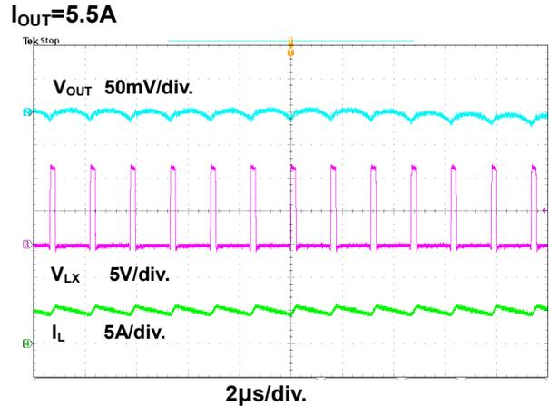
Figure 18. DC Ripple Waveform
