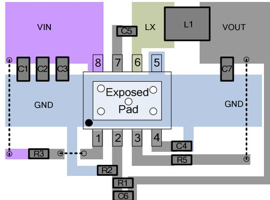
Figure 28. Recommended PCB Layout Diagram for SP Package
