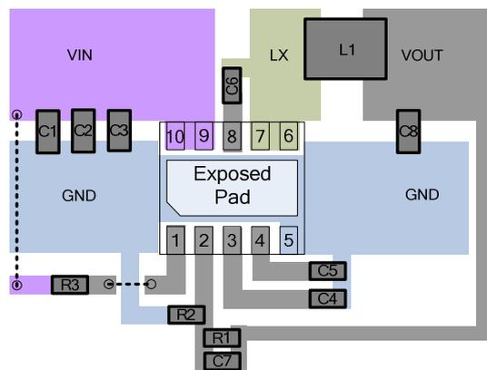
Figure 29. Recommended PCB Layout Diagram for DA Package
