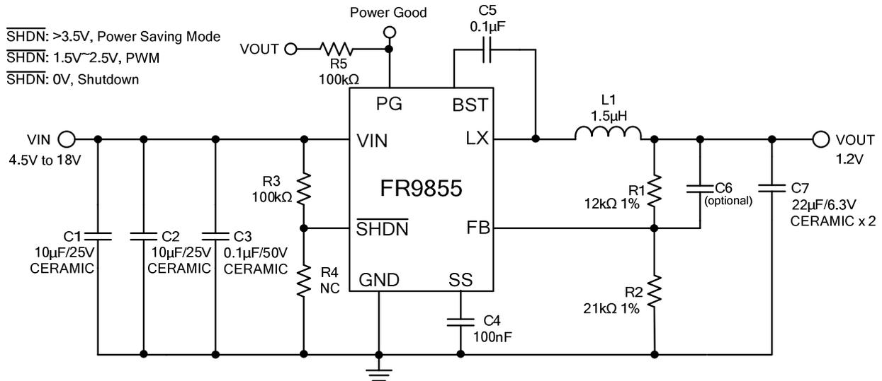
Figure 2. Application Circuit for SOP-8 Exposed Pad Package
