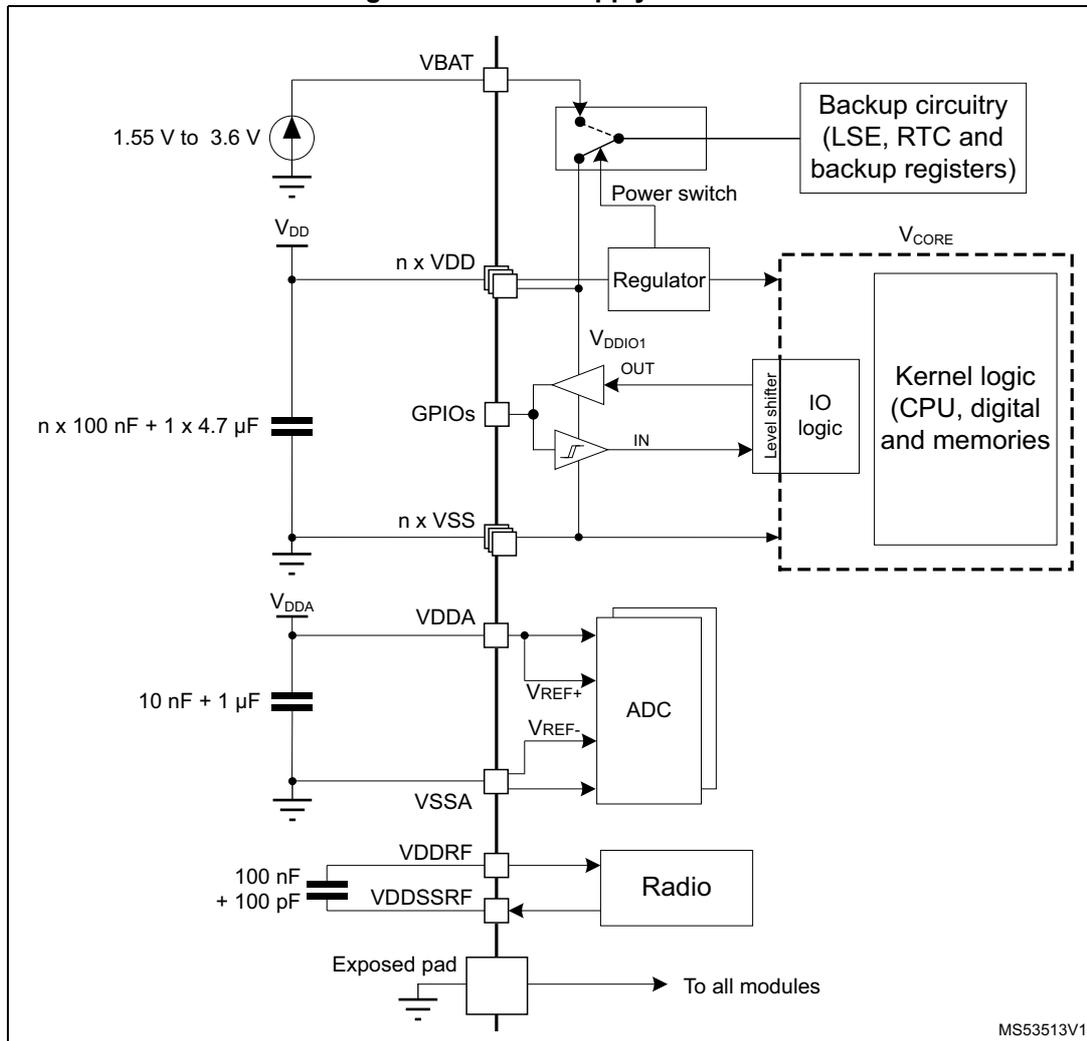
**Caution:** Each power supply pair ( $V_{DD} / V_{SS}$ ,  $V_{DDA} / V_{SSA}$  etc.) must be decoupled with filtering ceramic capacitors as shown in [Figure 10](#). These capacitors must be placed as close as possible to (or below) the appropriate pins on the underside of the PCB to ensure the good functionality of the device.
