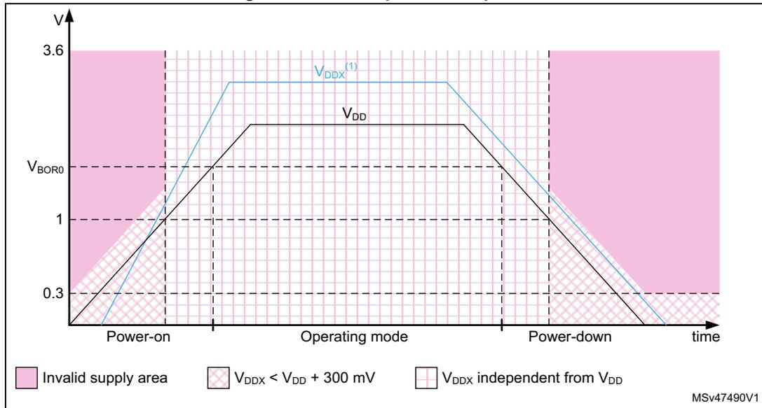
1.  $V_{DDX}$  refers to  $V_{DDA}$ .
