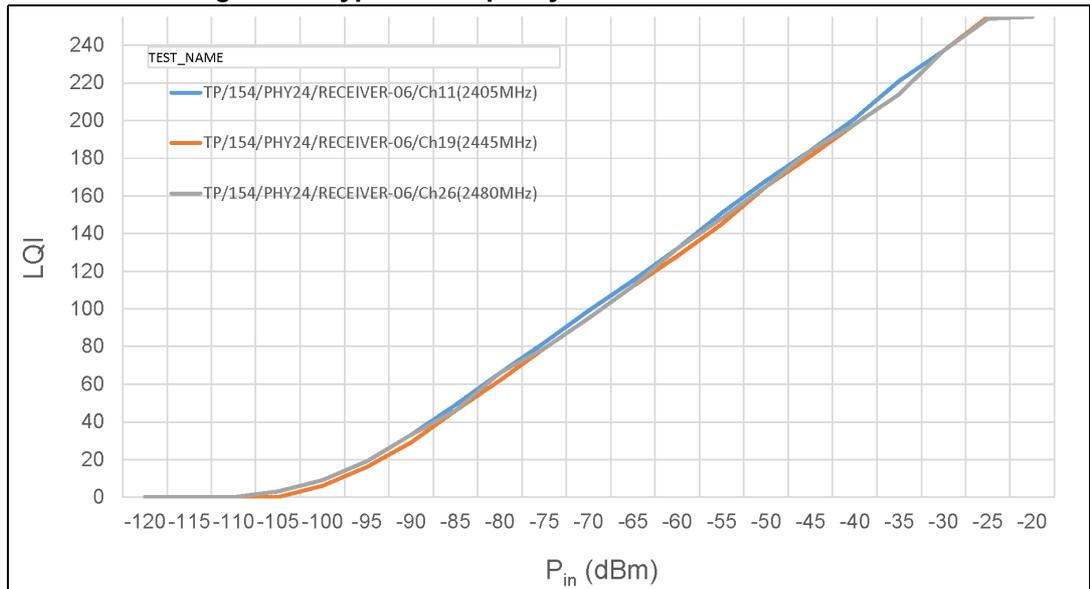
Figure 13. Typical energy detection (T = 27°C, V<sub>DD</sub> = 3.3 V)
