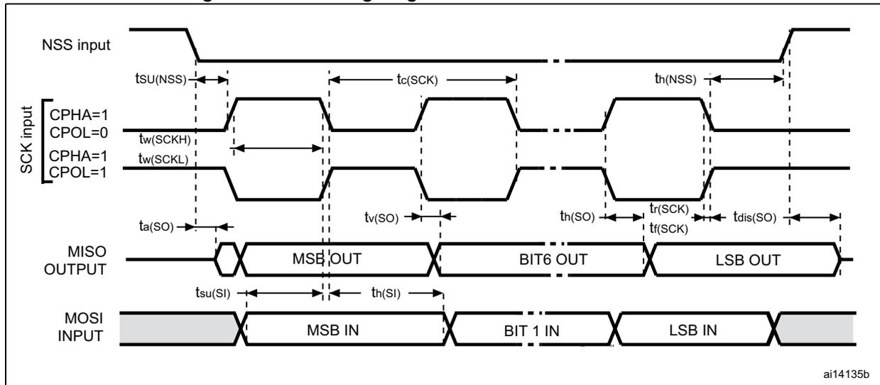
1. Measurement points are set at CMOS levels: 0.3 V<sub>DD</sub> and 0.7 V<sub>DD</sub>.
