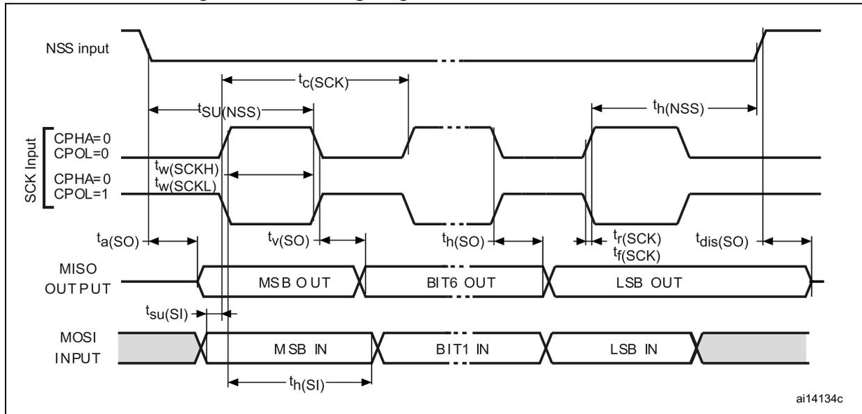
Figure 24. SPI timing diagram - slave mode and CPHA = 1
