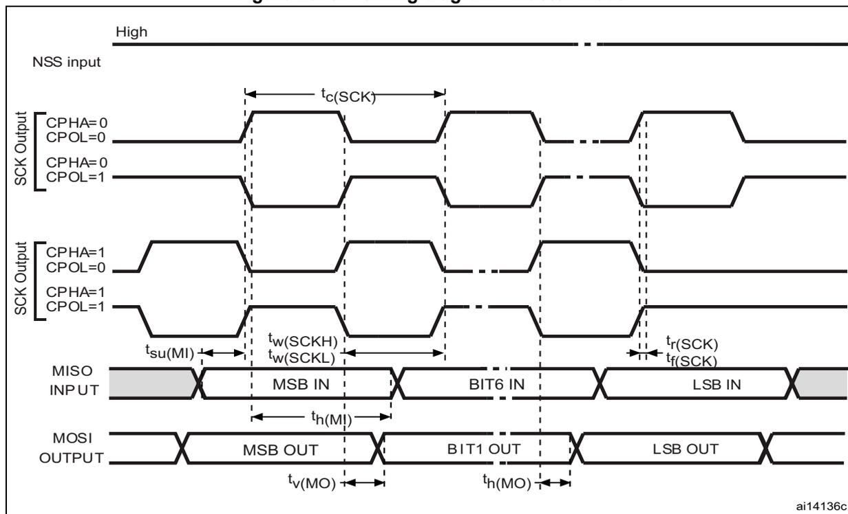
1. Measurement points are set at CMOS levels: 0.3  $V_{DD}$  and 0.7  $V_{DD}$ .
