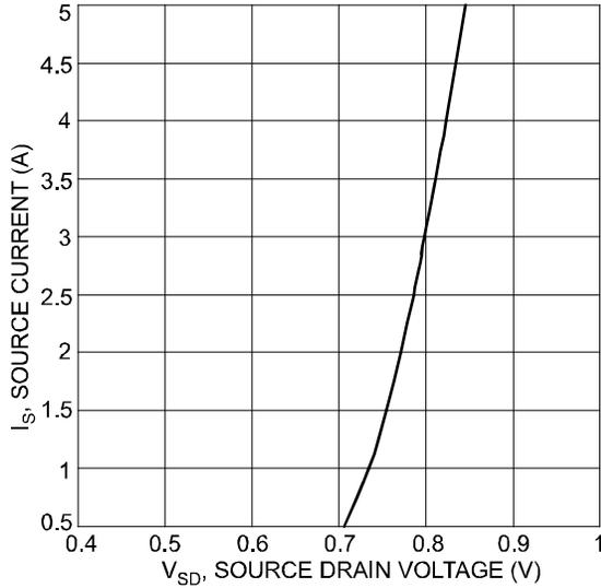
Fig. 7 Reverse Drain Current vs. Source-Drain Voltage
