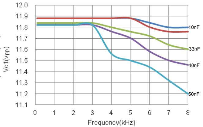
**Performance Characteristics** (Cont. @T<sub>A</sub> = +25°C, V<sub>IN</sub> = 3.0V, C<sub>Piezo</sub> = 15nF, f<sub>DIN</sub> = 4kHz, unless otherwise specified.)
