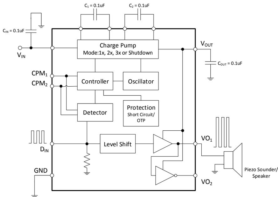
When using the PAM8904Q with a single ended output, the  $VO_2$  pin should be left open circuit.
