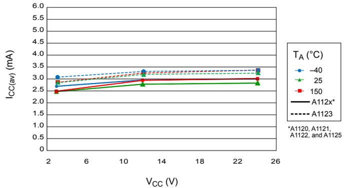
Average Supply Current (Off) versus Ambient Temperature
