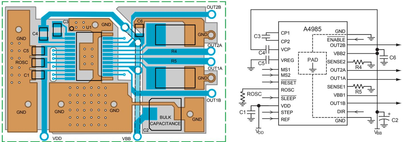
Figure 9: LP Package Typical Application and Circuit Layout
