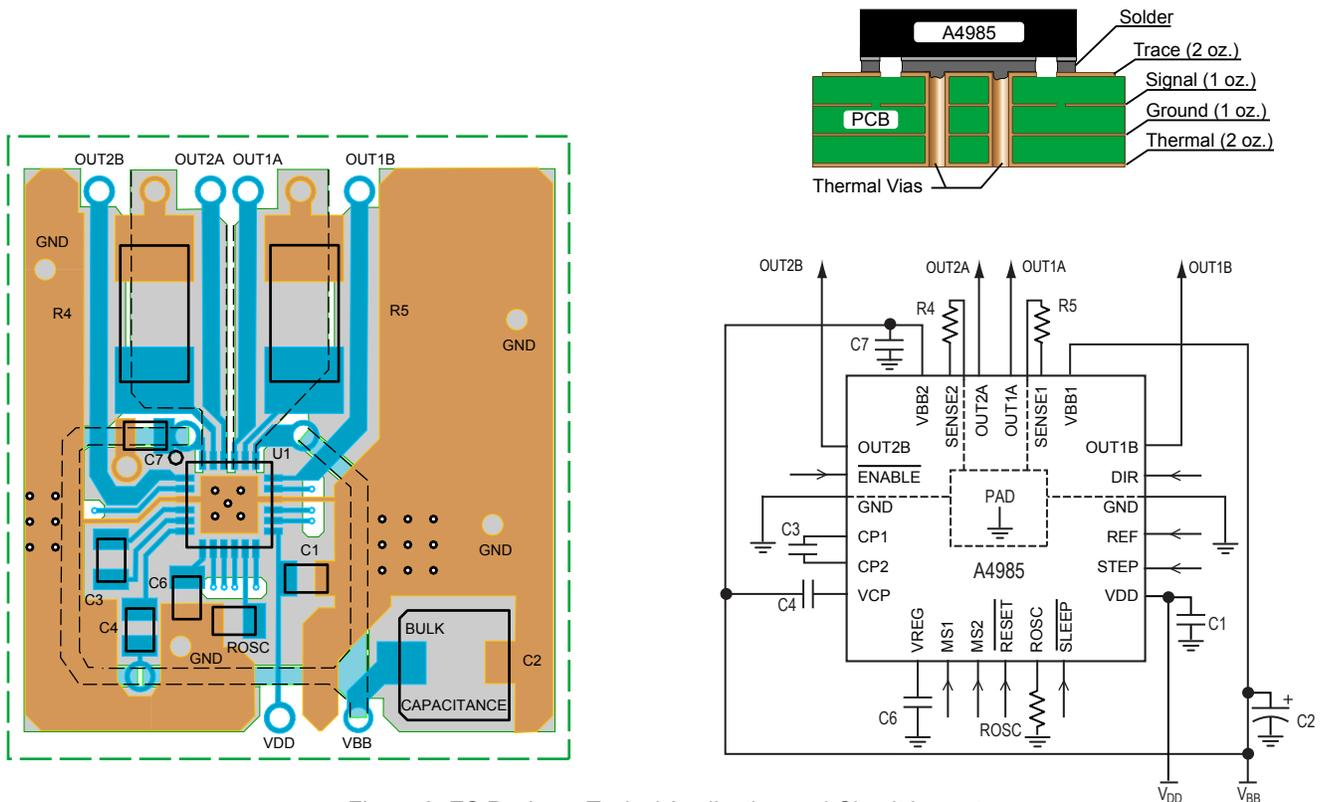
Figure 8: ES Package Typical Application and Circuit Layout
