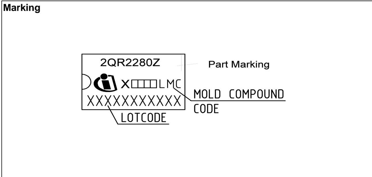
Figure 14 Marking for ICE2QR2280Z
