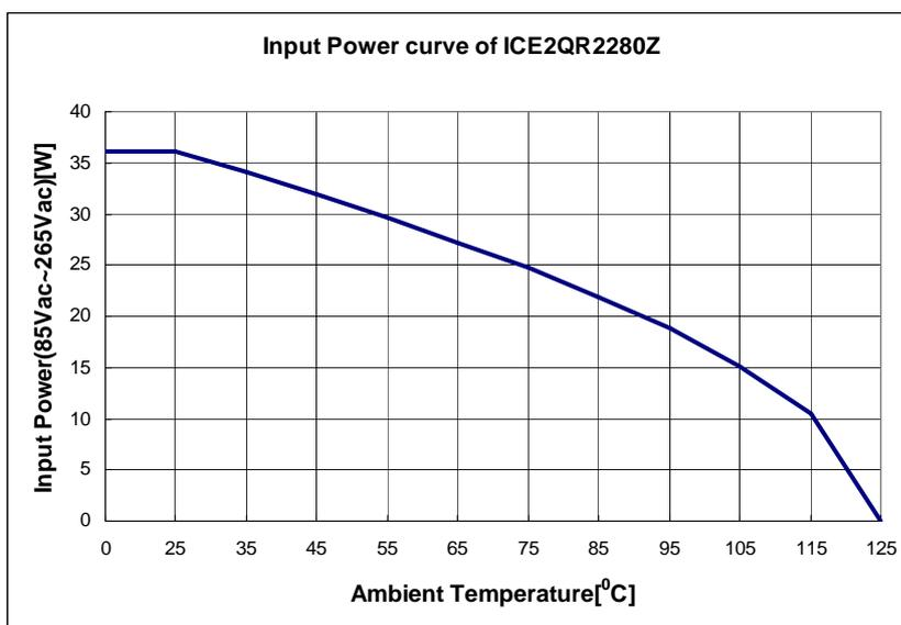
Figure 12 Input Power curve  $V_{in}=230V_{ac}$ ;  $P_{in}=f(T_a)$
