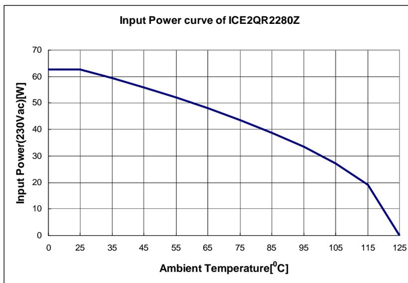
Figure 11 Input Power curve  $V_{in}=85\sim 265V_{ac}$ ;  $P_{in}=f(T_a)$
