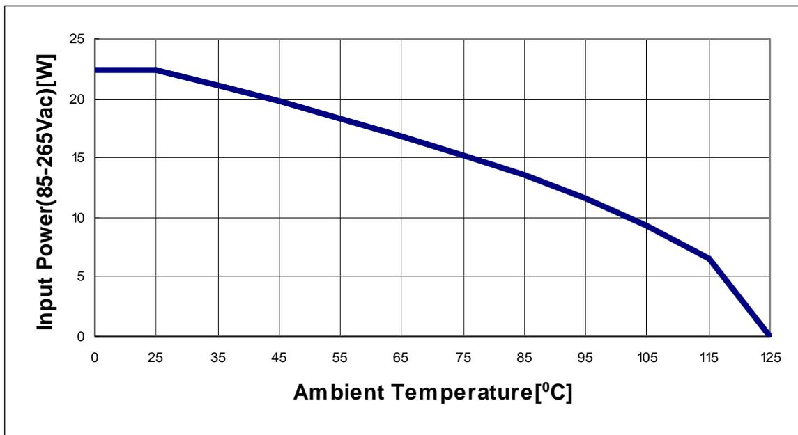
Figure 12 Input Power curve  $V_{in}=85\sim 265\text{Vac}$ ;  $P_{in}=f(T_a)$
