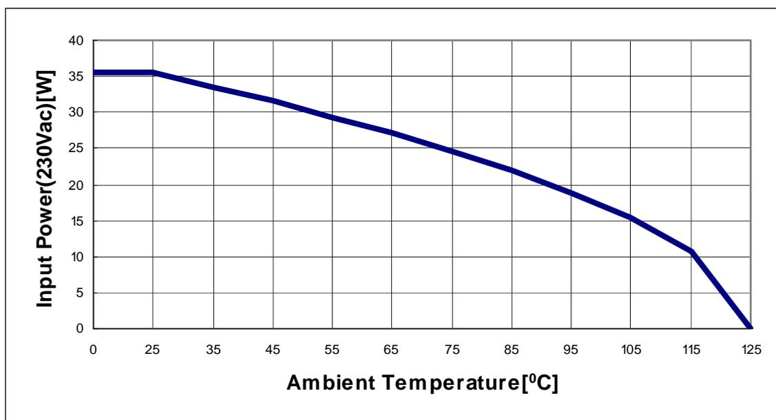
Figure 13 Input Power curve  $V_{in}=230\text{Vac}$ ;  $P_{in}=f(T_a)$
