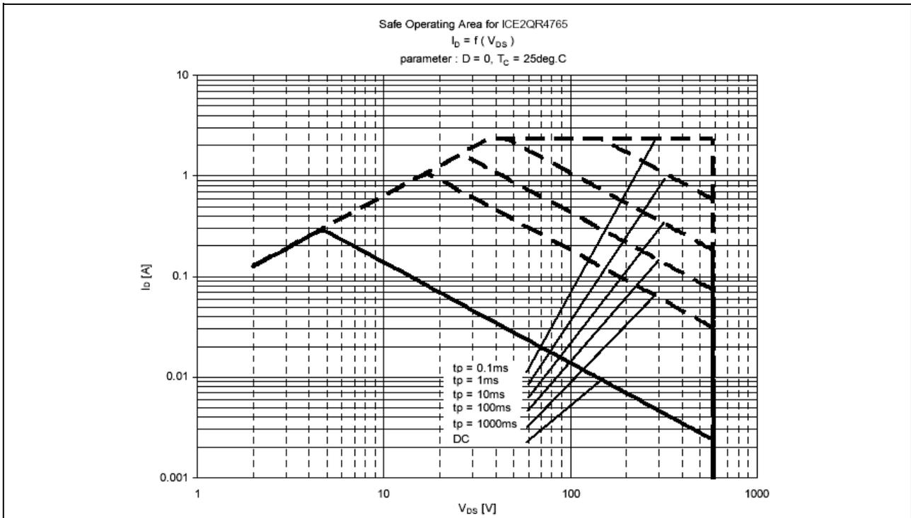
Figure 9 Safe Operating Area(SOA) curve for ICE2QR4765
