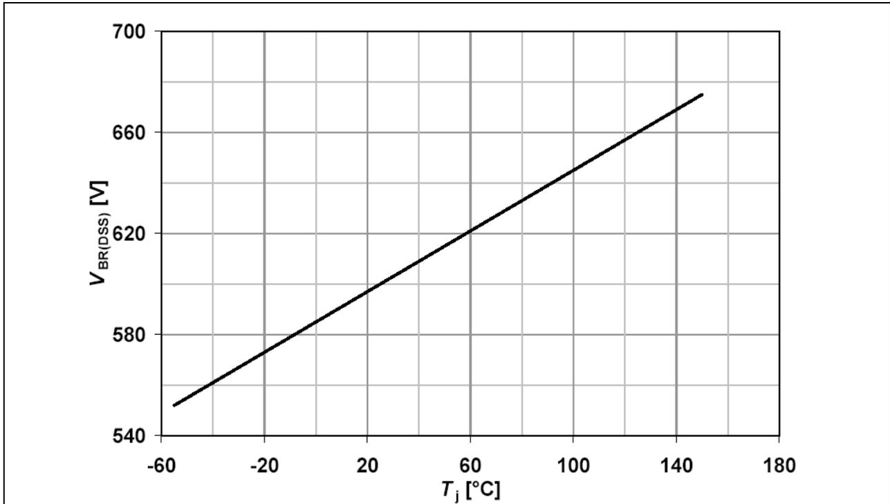
Figure 11 Drain-source breakdown voltage;  $V_{BR(DSS)}=f(T_j)$
