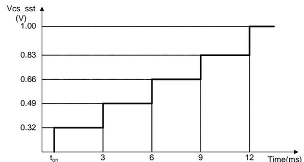
Figure 4 Maximum current sense voltage during softstart
