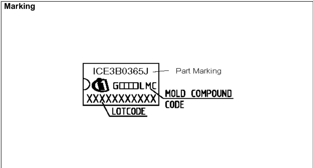
Figure 24 Marking for ICE3B0365J
