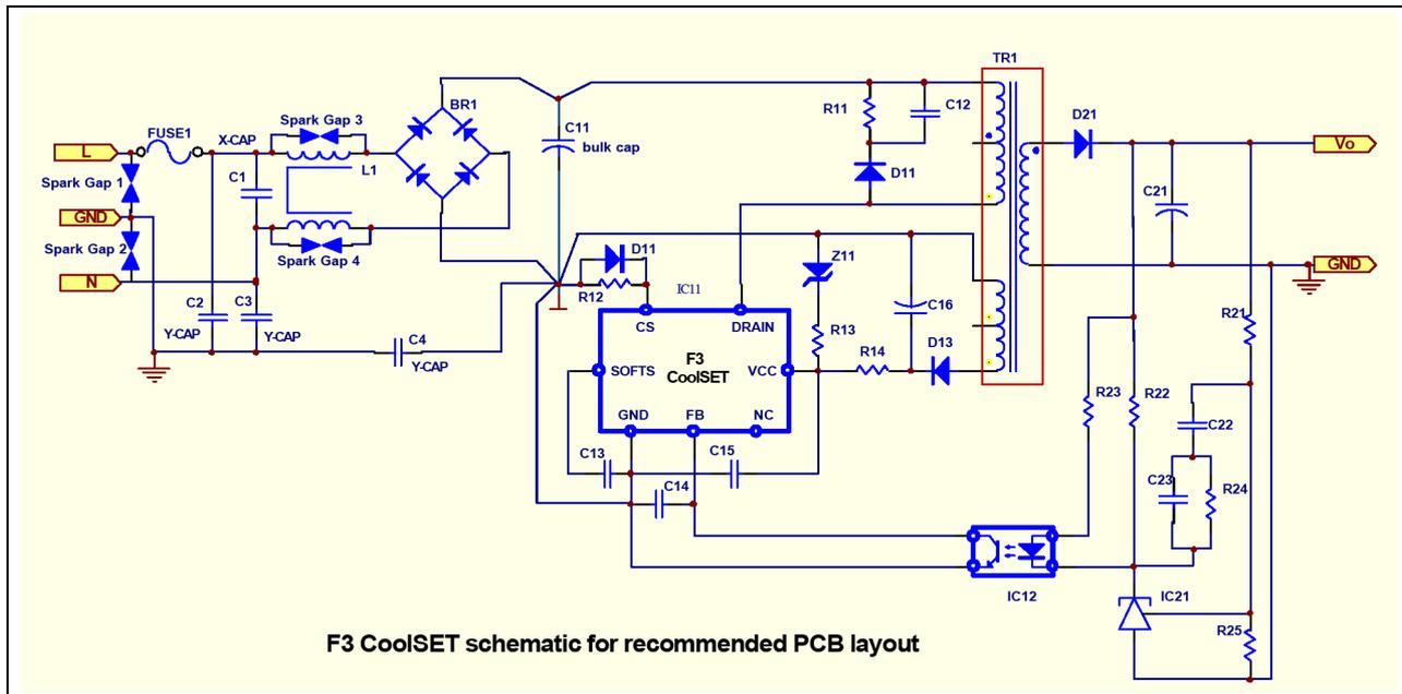
Figure 28 Schematic for recommended PCB layout
