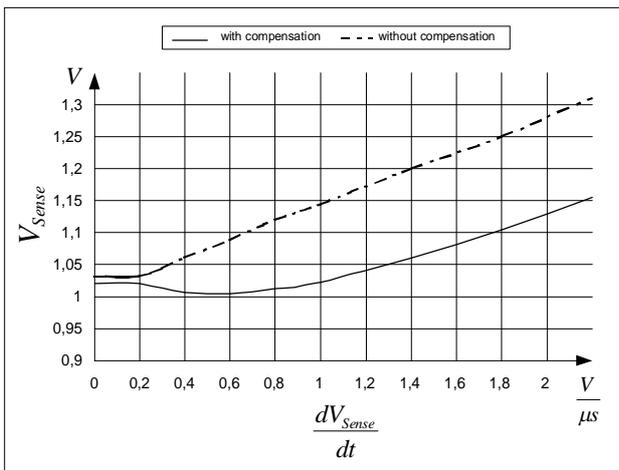
Figure 11 Overcurrent Shutdown
