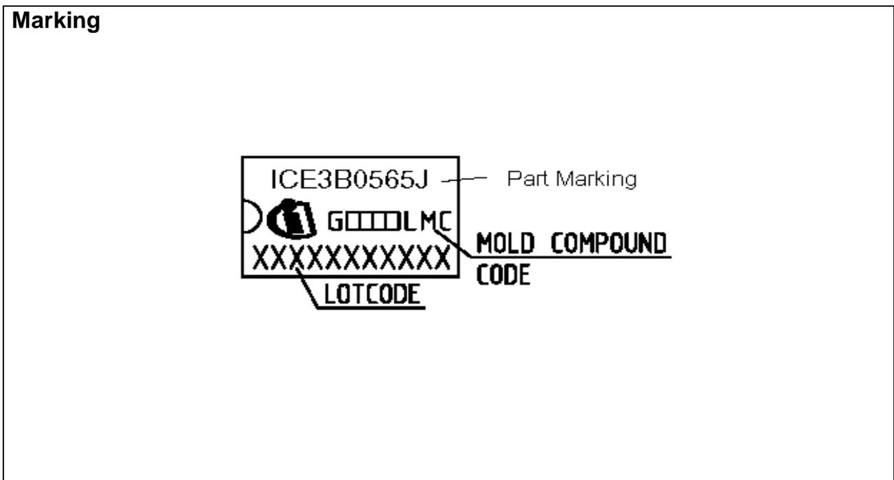
Figure 25 Marking for ICE3B0565J
