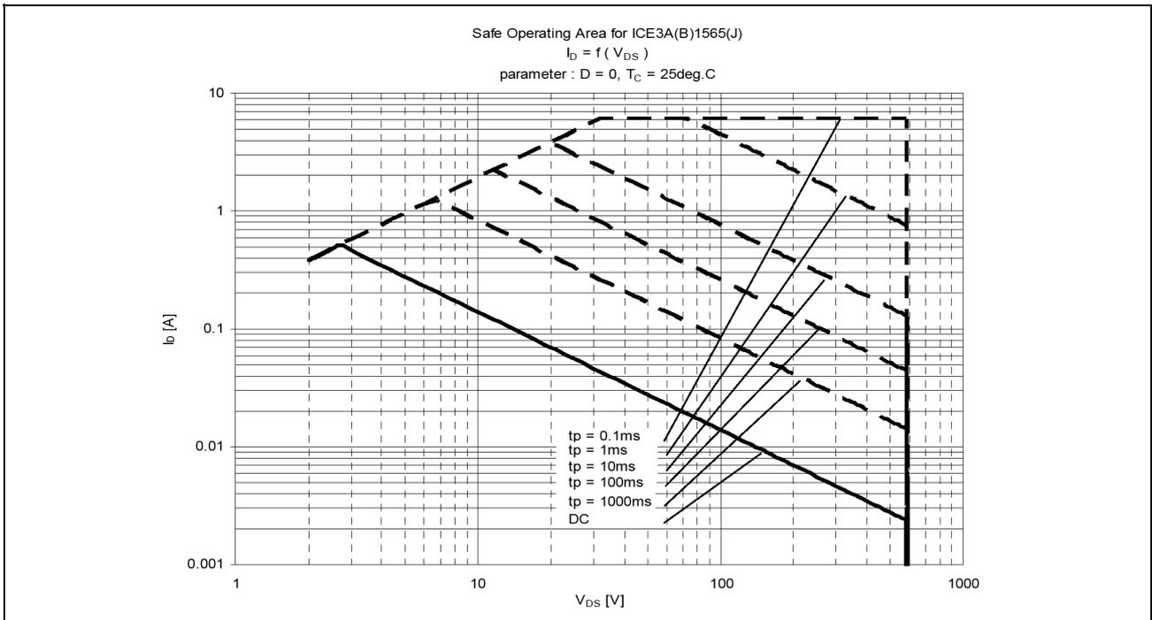
Figure 20 Safe Operating area ( SOA ) curve for ICE3B1565J
