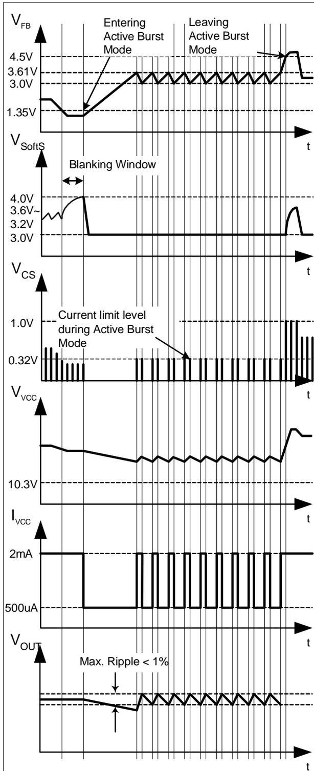
Figure 15 Signals in Active Burst Mode
