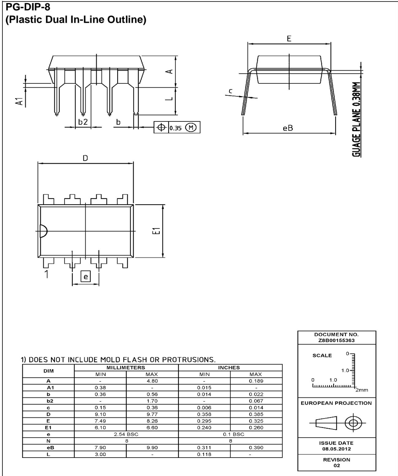
Figure 23 PG-DIP-8 ( Pb-free lead plating Plastic Dual-in-Line Outline )
