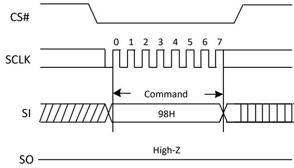
**Figure 32a. The Global Block/Sector Unlock Sequence Diagram (QPI)**
