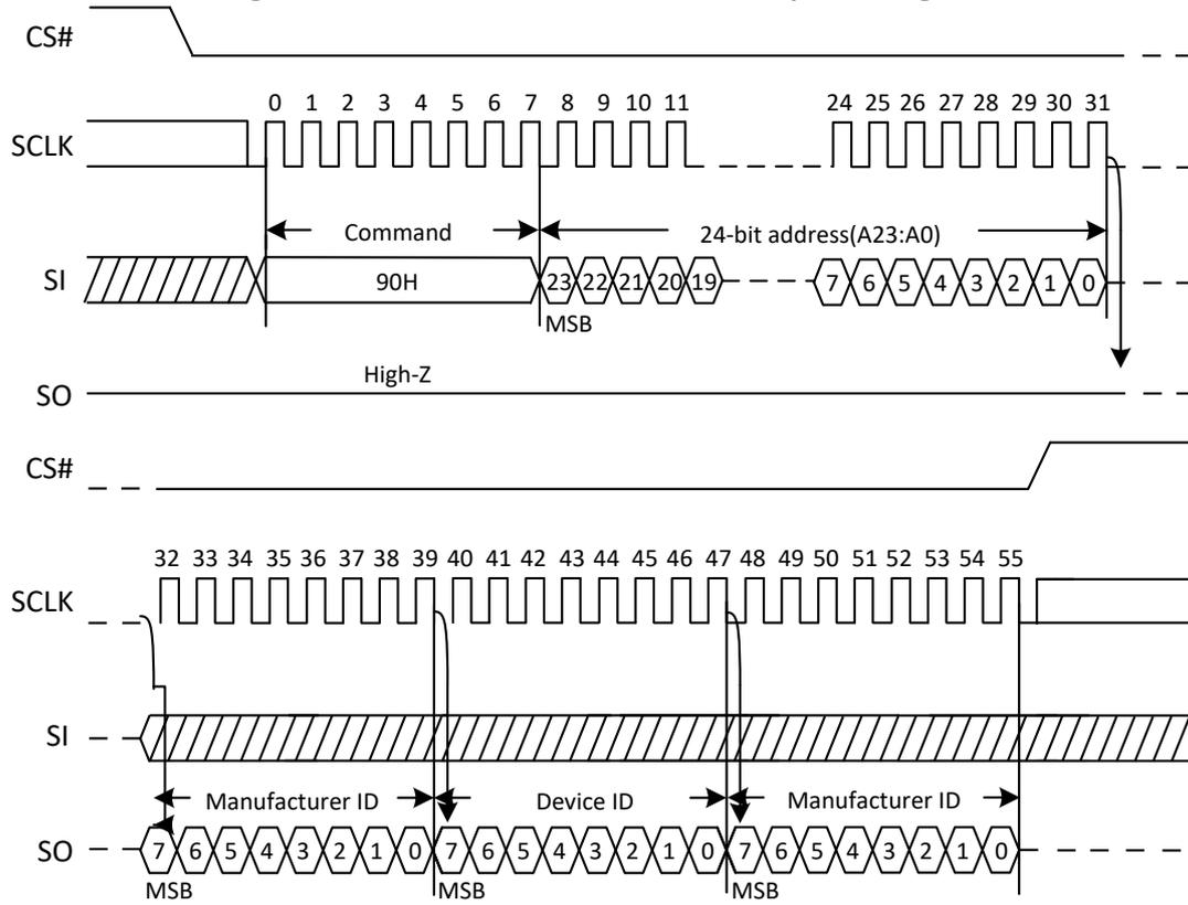
Figure27a. Read Manufacture ID/ Device ID Sequence Diagram (QPI)
