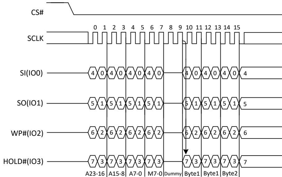
**Quad I/O Word Fast Read with “8/16/32/64-Byte Wrap Around” in Standard SPI mode**
