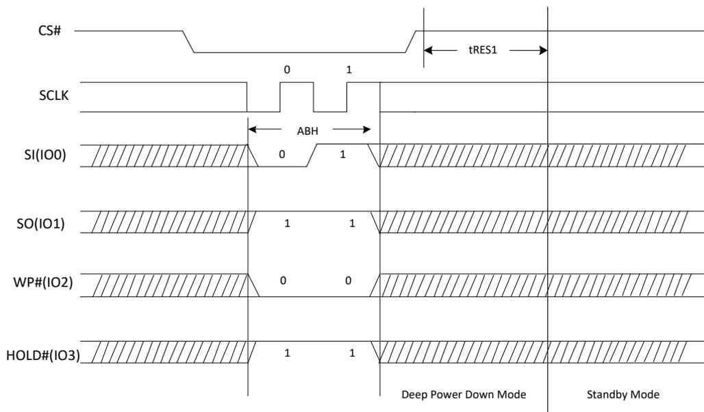
Figure26. Release Power-Down/Read Device ID Sequence Diagram
