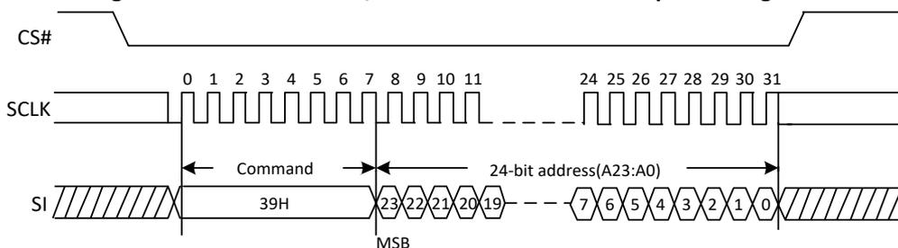
**Figure 33c. Individual Block/Sector Unlock command Sequence Diagram (QPI)**
