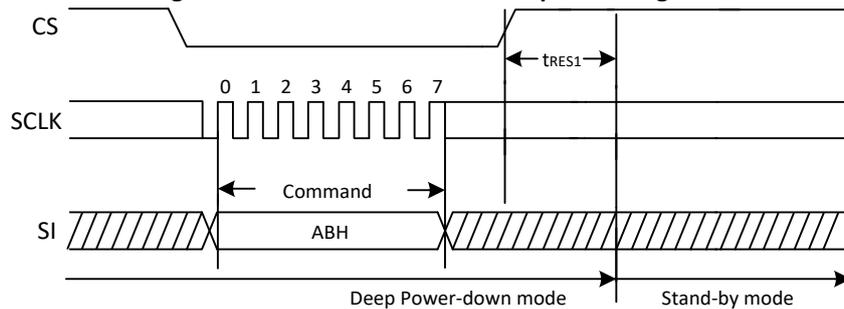
**Figure25a. Release Power-Down Sequence Diagram (QPI)**
