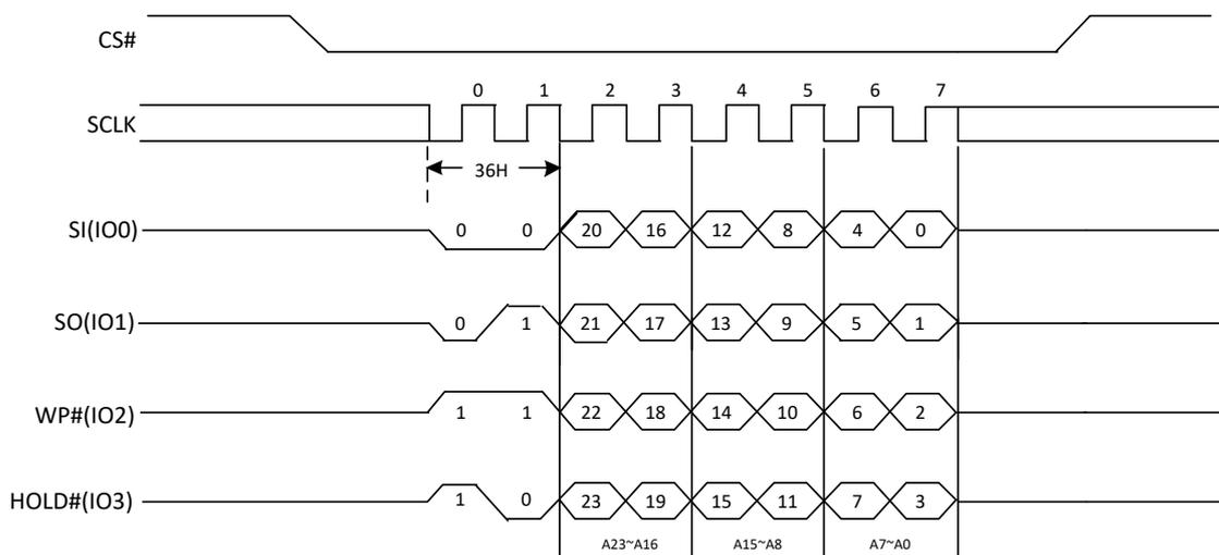
**Figure33b. Individual Block/Sector Unlock command Sequence Diagram**
