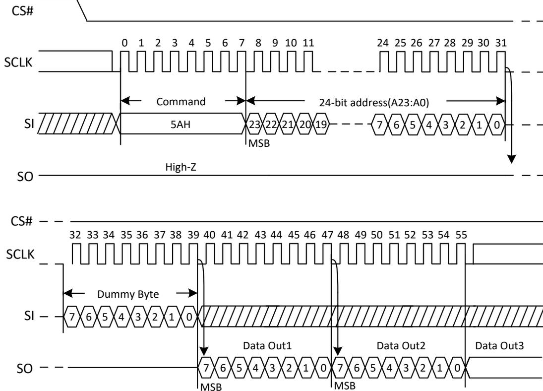
**Figure42b. Read Serial Flash Discoverable Parameter command Sequence Diagram (QPI)**
