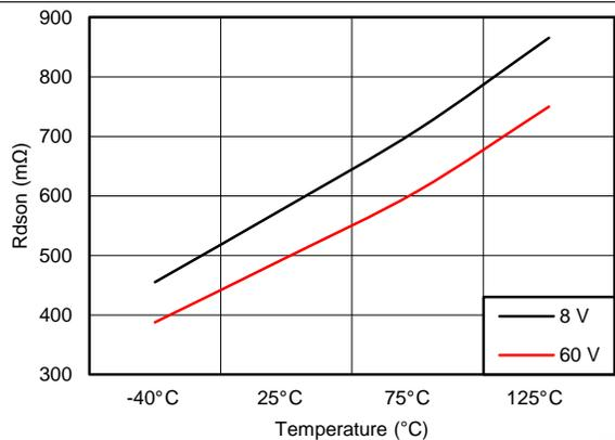
Figure 4.  $R_{DS(on)}$  Over Temperature
