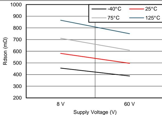
Figure 5.  $R_{DS(on)}$  Over  $V_M$
