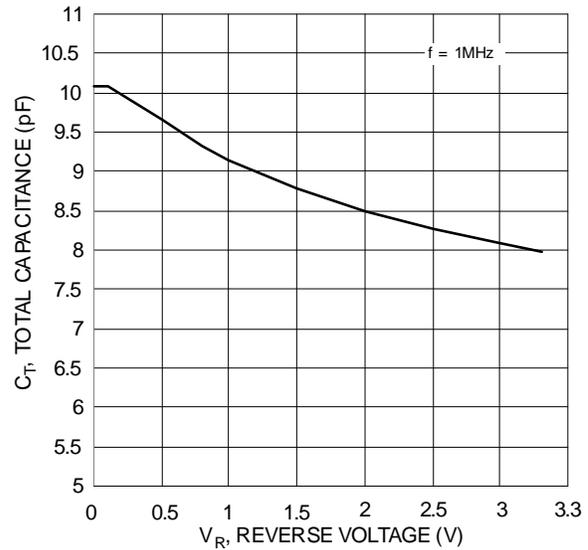
Figure 2 Typical Capacitance
