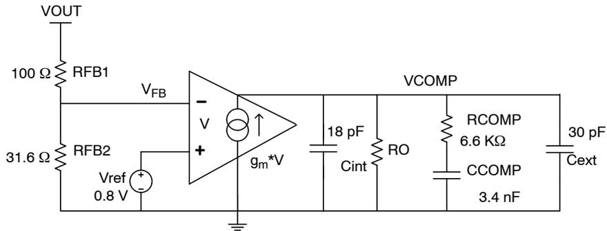
Figure 31. Example of the Feedback Compensation Network
