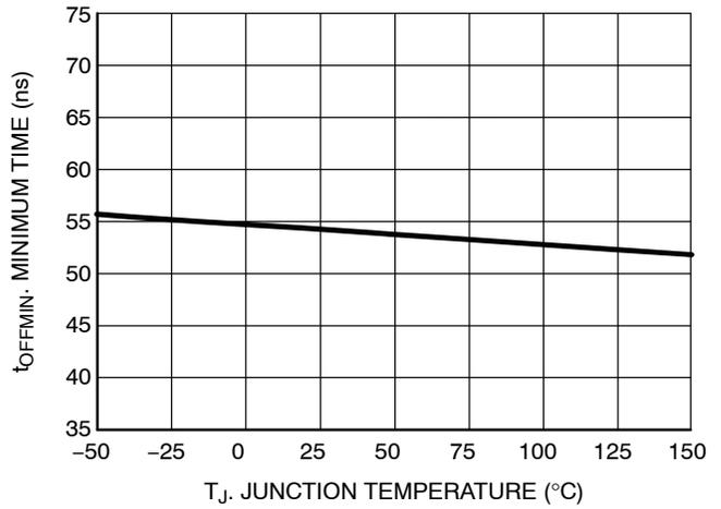
Figure 17. Minimum Off Time vs. Junction Temperature
