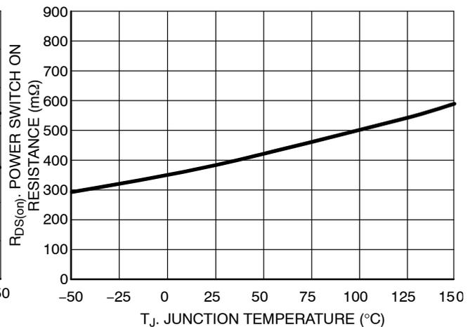
Figure 15. Power Switch  $R_{DS(on)}$  vs. Junction Temperature
