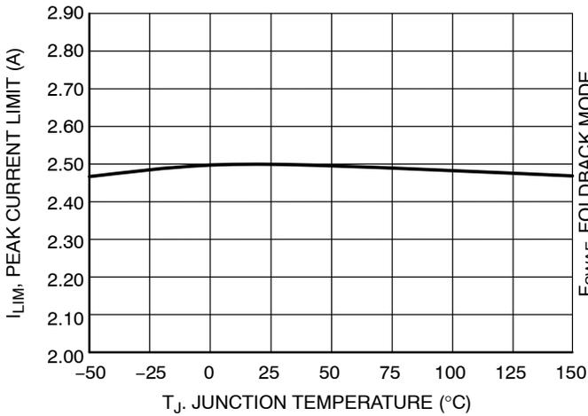
Figure 18. Current Limit Threshold vs. Junction Temperature
