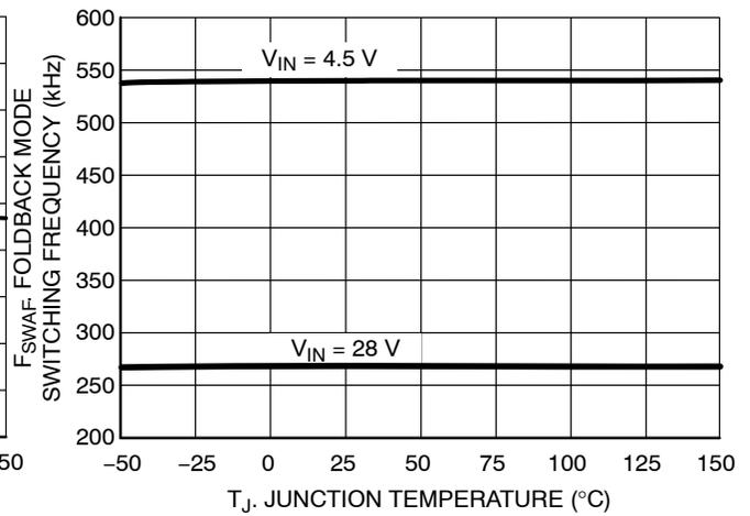
Figure 19. Short-Circuit Foldback Frequency vs. Junction Temperature
