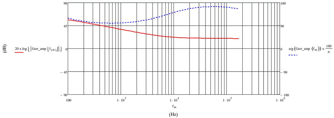
Figure 32. Bode Plot of the OTA Compensator
