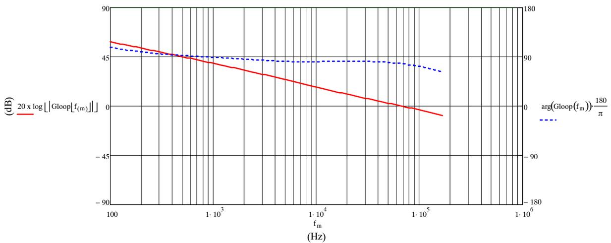
Figure 33. Bode Plot of the Total Loop
