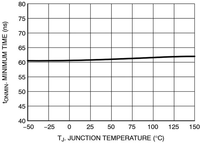
Figure 16. Minimum On Time vs. Junction Temperature
