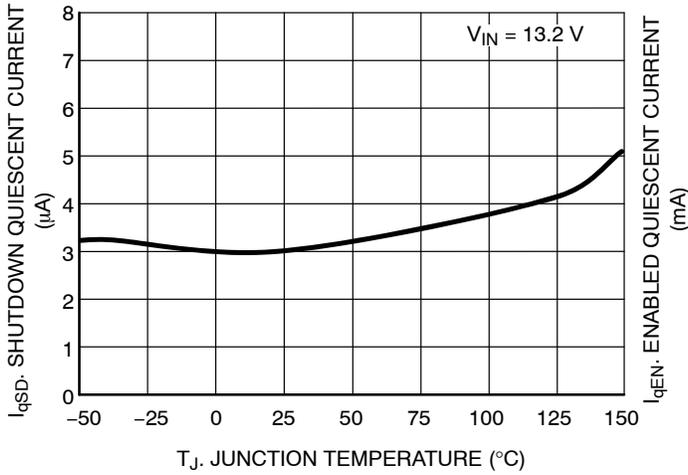
Figure 4. Shutdown Quiescent Current vs. Junction Temperature
