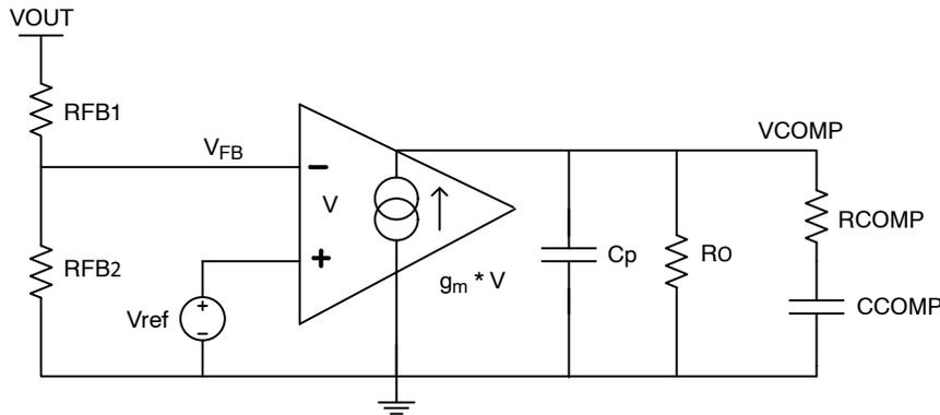
Figure 29. Feedback Compensator Network Model
