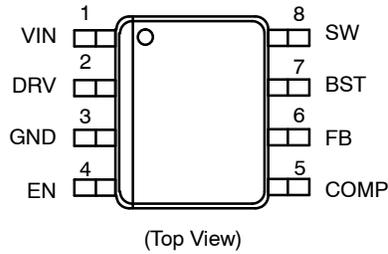
**Figure 3. Pin Connections**
