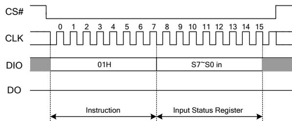
Figure 7.4 Write Status Register Instruction Sequence Diagram
