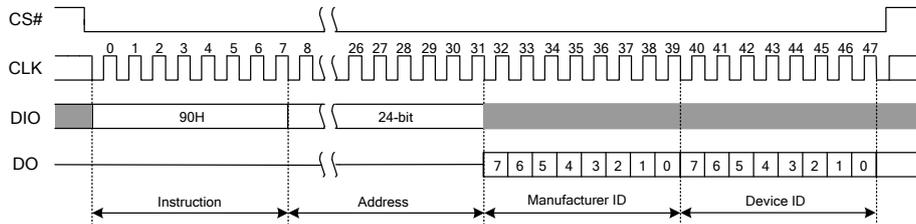
Figure 7.14 Read Manufacturer / Device ID Diagram
