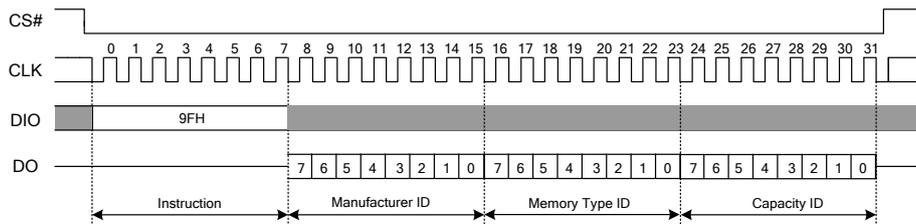
Figure 7.15 Read JEDEC ID instruction Sequence Diagram
