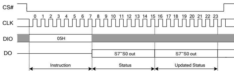
Figure 7.3 Read Status Register Instruction Sequence Diagram
