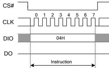
Figure 7.2 Write Disable Instruction Sequence Diagram
