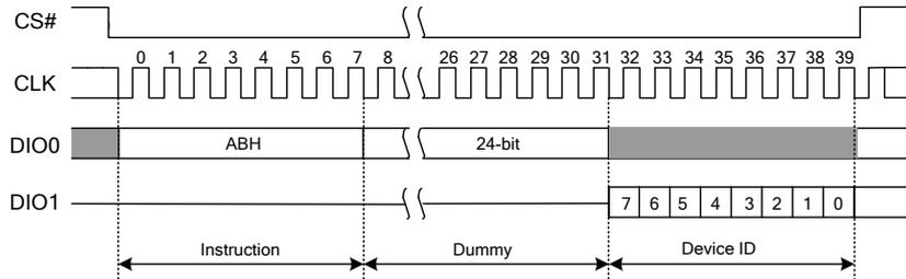
Figure 7.13 Release Power-down / Device ID Instruction Sequence Diagram
