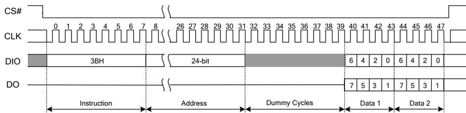
Figure 7.7 Fast Read Dual Output Instruction Sequence Diagram
