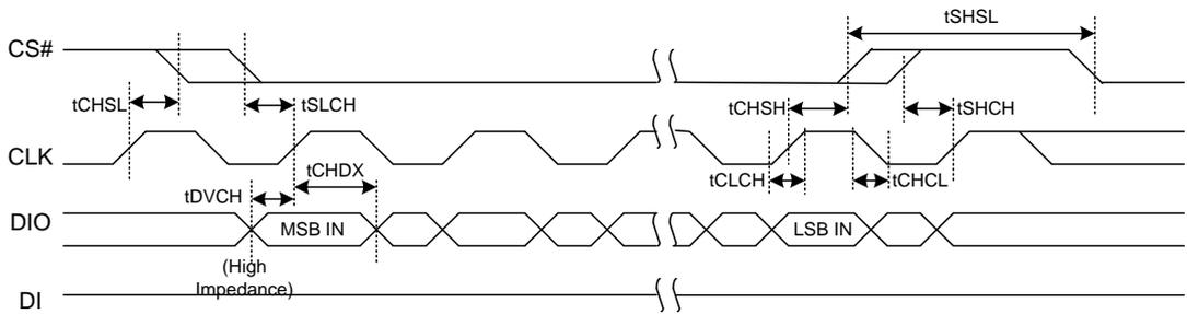
Figure 8.4 Input Timing
