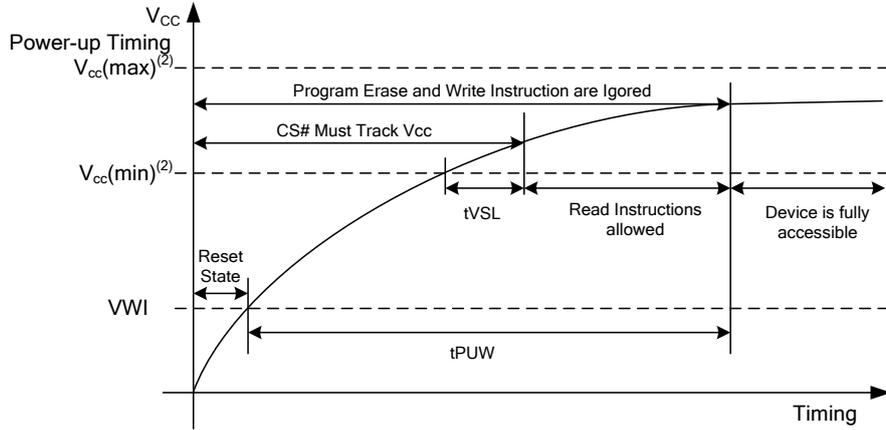
Figure 8.1 Power-up Timing
