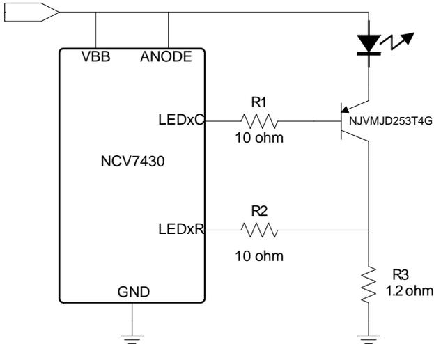
Figure 12. Using the NCV7430 with Higher Current LEDs
