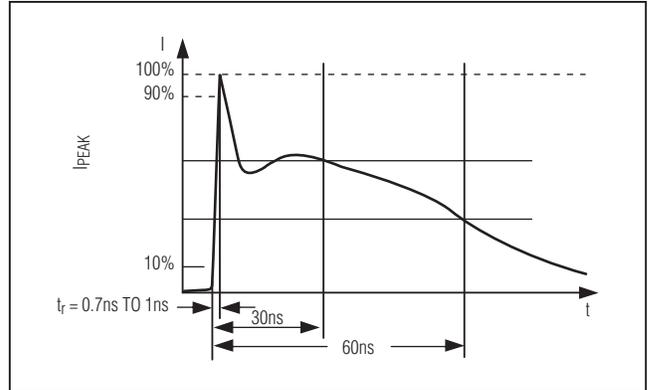
Figure 10d. IEC 61000-4-2 ESD Generator Current Waveform
