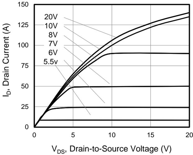
Figure 2. Transfer Characteristics
