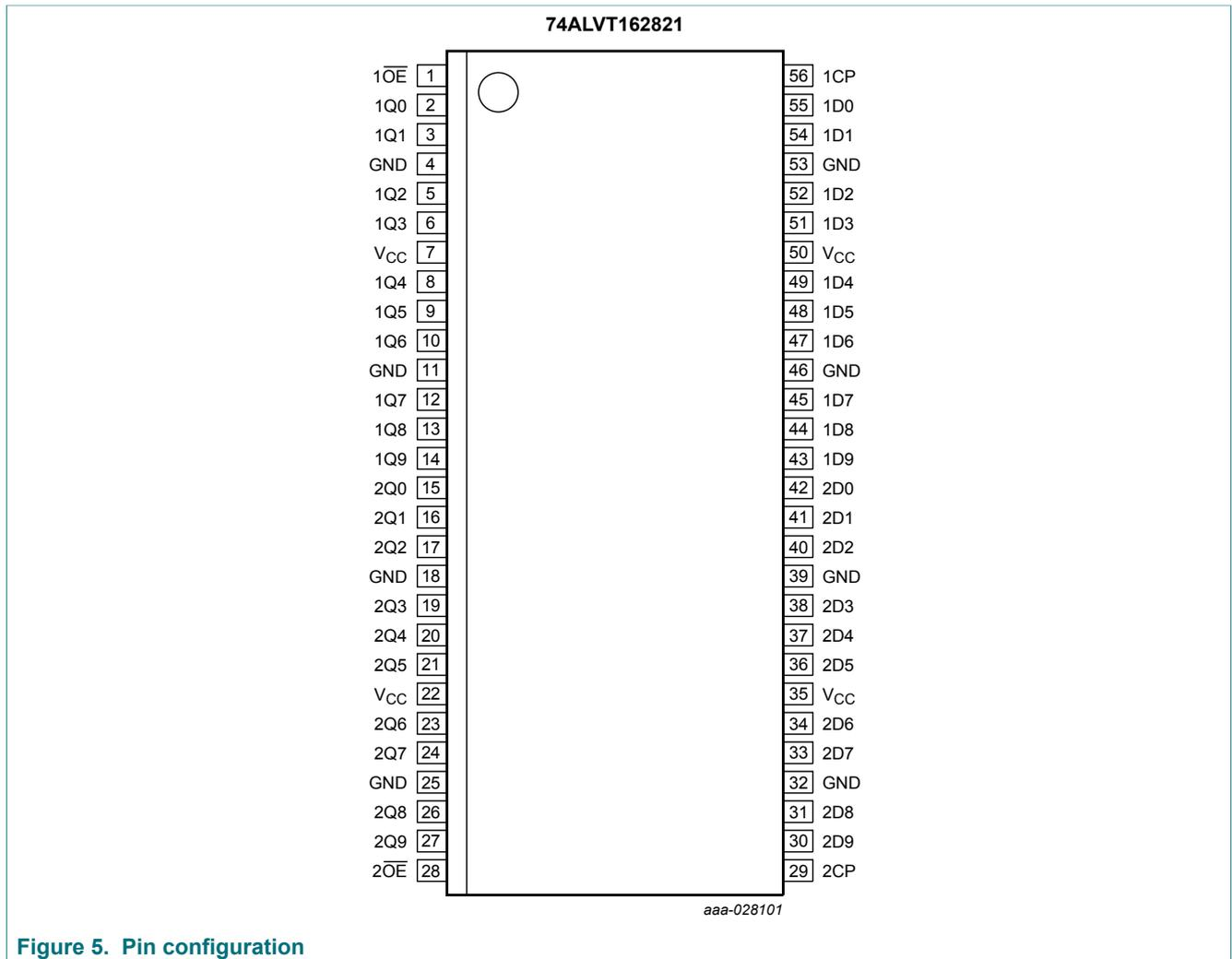
Figure 5. Pin configuration
