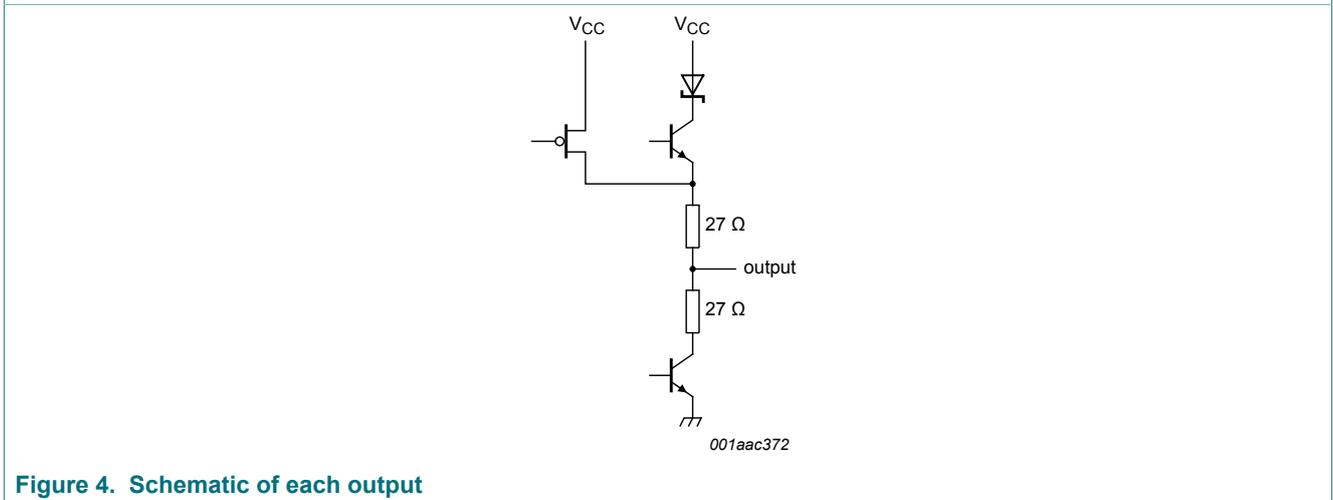
Figure 4. Schematic of each output
