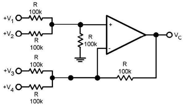
Where:  $V_O = V_1 + V_2 - V_3 - V_4$ ,  $(V_1 + V_2) \geq (V_3 + V_4)$  to keep  $V_O > 0$   $V_{DC}$
