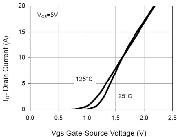
Figure 5 Transfer Characteristics
