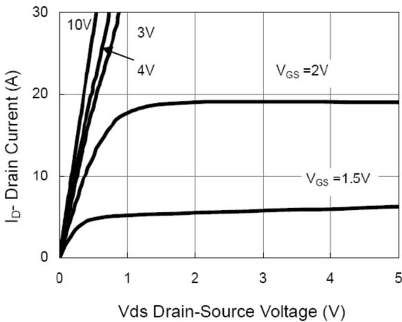
Figure 3 Output Characteristics
