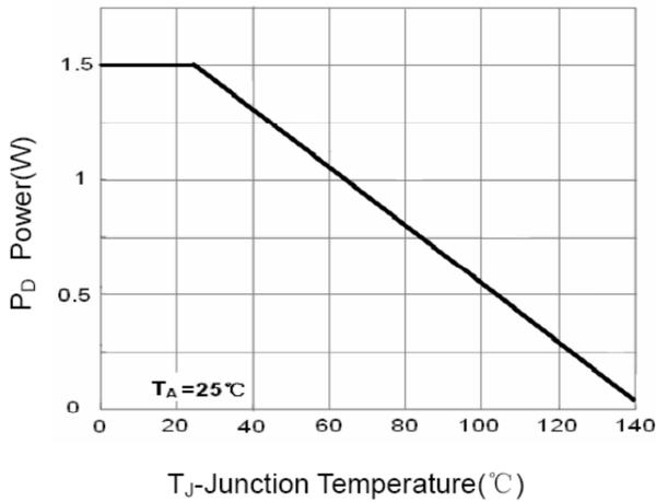
Figure 1 Power Dissipation
