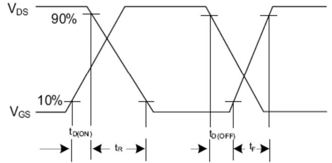
Fig. 2.2 Switching Waveforms
