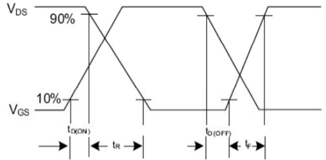
Fig. 2.2 Switching Waveforms
