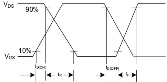
Fig. 2.2 Switching Waveforms
