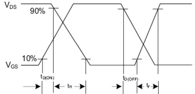
Fig. 2.2 Switching Waveforms
