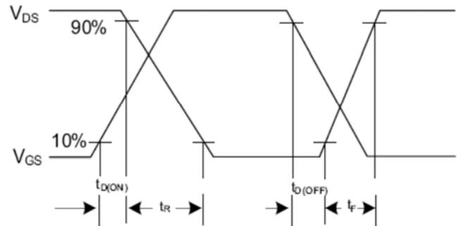
Fig. 2.2 Switching Waveforms
