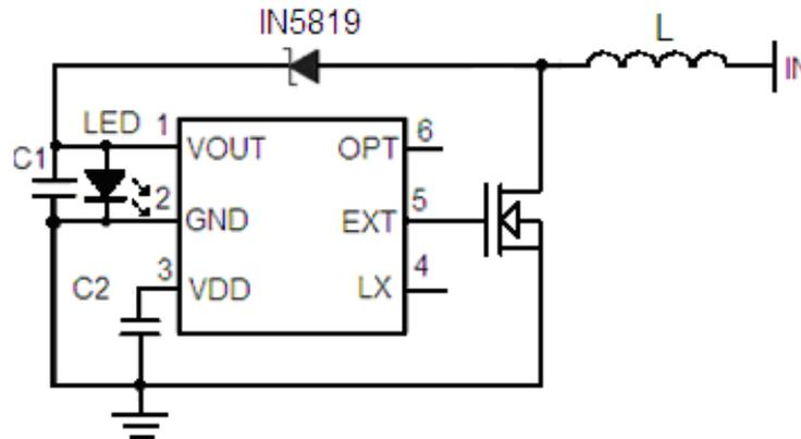
Figure1 without expending output current MOSFET's application (one or two dry batteries)
