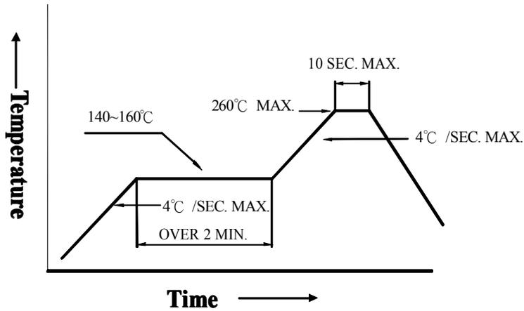
3. DIP soldering (Wave Soldering) :
